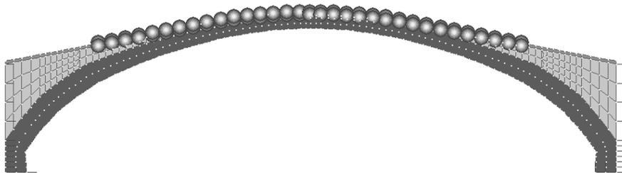
Fig. 5 Bridge with non-structural masses representing stone parapets.
