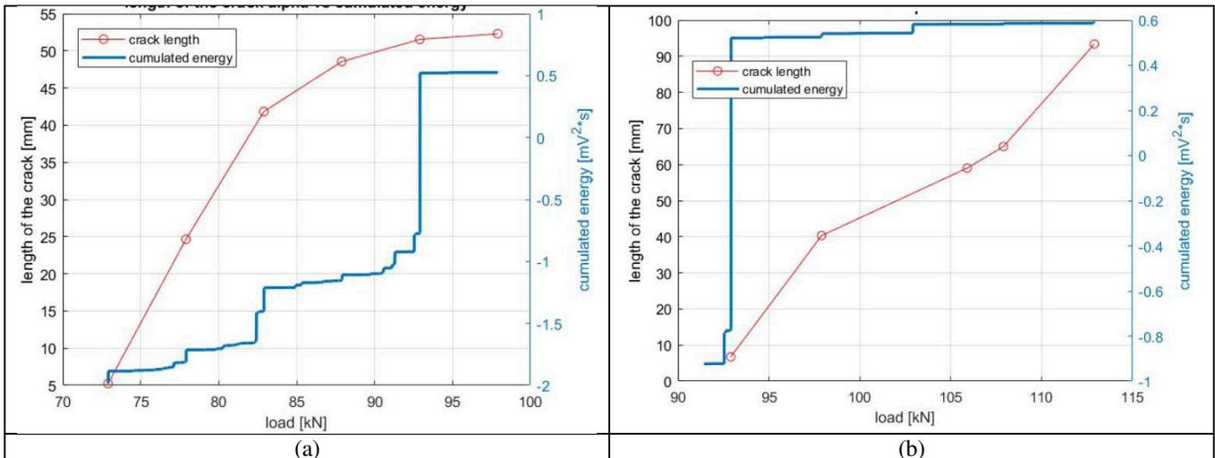
**Fig. 9** Crack length and cumulated energy (in logarithmic scale) vs. load: for the two cracks shown in Fig. 7.
