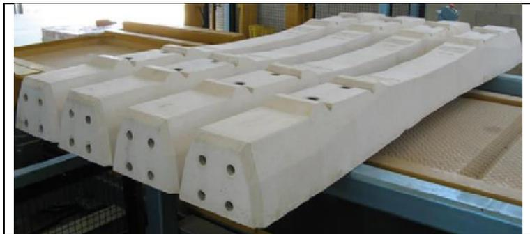
Fig. 1 Examples of prestressed railway sleepers.
