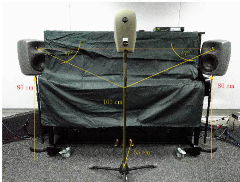
Figure 5. Upright piano recording setup.
