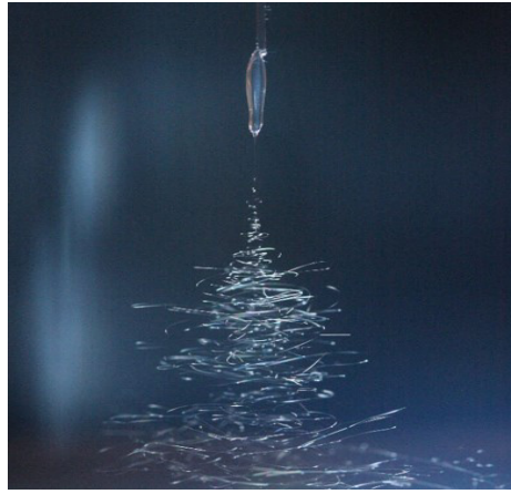
Figure 7: Electrospinning of PLA under optimal conditions
