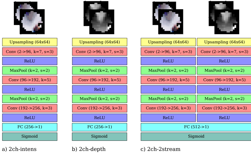
Figure 4: Network structures used: a) U(64) - C(2 \rightarrow 96, k=7, s=3) - \text{ReLU} - P(k=2, s=2) - C(96 \rightarrow 192, k=5, s=1) - \text{ReLU} - P(k=2, s=2) - C(192 \rightarrow 256, k=3, s=1) - \text{ReLU} - F(256 \rightarrow 1) - \text{Sigmoid} , b) same structure as a) but input with depth images. c) Two branches U(64) - C(2 \rightarrow 96, k=7, s=3) - \text{ReLU} - P(k=2, s=2) - C(96 \rightarrow 192, k=5, s=1) - \text{ReLU} - P(k=2, s=2) - C(192 \rightarrow 256, k=3, s=1) - \text{ReLU} , joined with F(512 \rightarrow 1) - \text{Sigmoid} , Notation : U(N) is the initial up-sampling to size N \times N C(i \rightarrow n, k=k, s=s) is a convolutional layer with i input channels, n filters of spatial size k \times k applied with stride s , P(k=k, s=s) is a max-pooling layer of size k \times k applied with stride s , and F(i \rightarrow n) denotes a fully connected linear layer with i input units and n output units.
