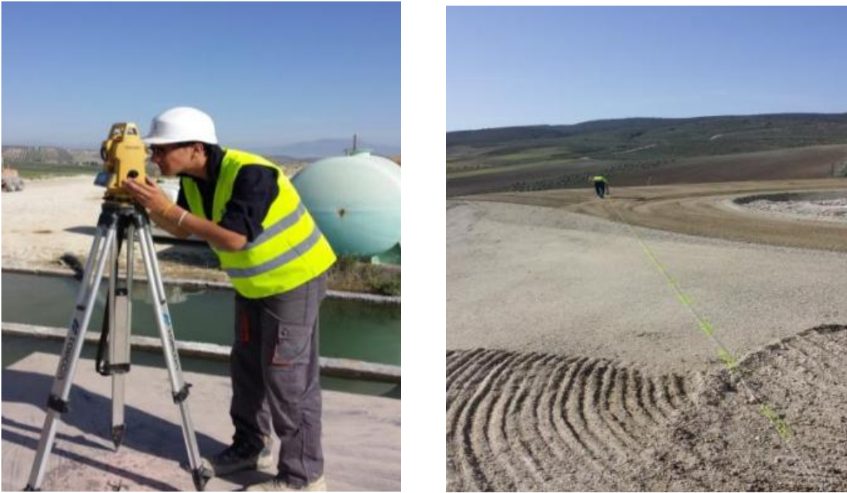
Figure 50. Perimeter measurement with a total station
