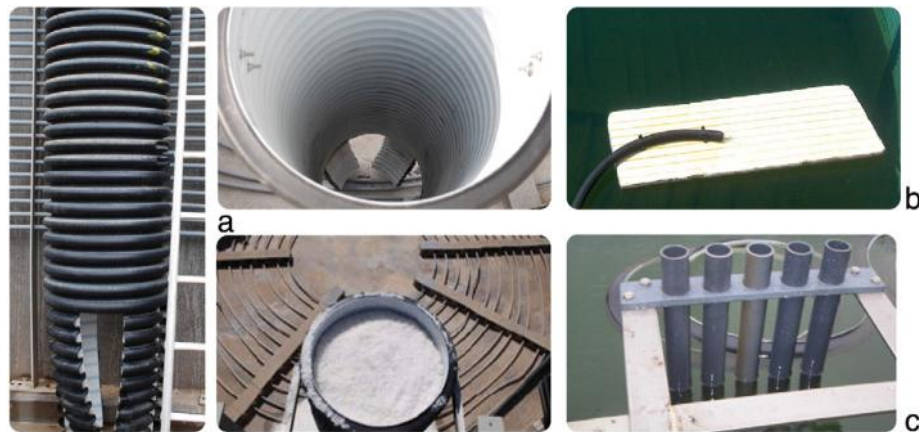
Figure 15. Maintenance equipment of salinity gradient: a) salt charger; b) fresh water supply system; c) control pH system
