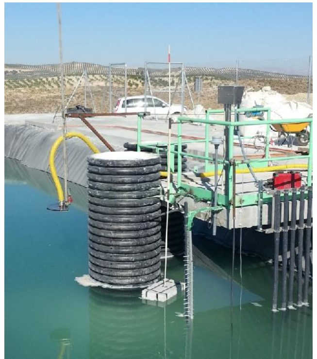
Figure 79. Salt charger, temperature sensors, system of pipes and diffusor on the catwalk
