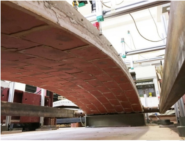
Fig. 9. Photo of one of the full-scale prototypes. View of the intrados showing the tile vault's pattern.
