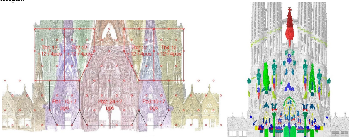
Figure 2. Distribution and zoning of the façade for the taking of data in detail, Left planning of data collection on the façade, right classification of sculptures in the planning of auxiliary positions
