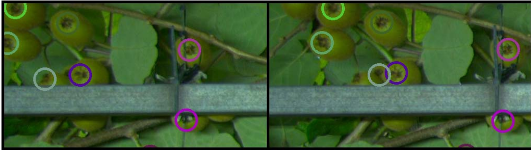
Fig. 6. Example of an incorrectly matched fruit. The match marked in gray is not the same fruit in both images. There are three fruit in a cluster with the middle fruit being partially occluded by the other two. All three of the fruit were detected in the right image, but the middle fruit was missed in the left image. The missed detection resulted in the wrong match being found.
