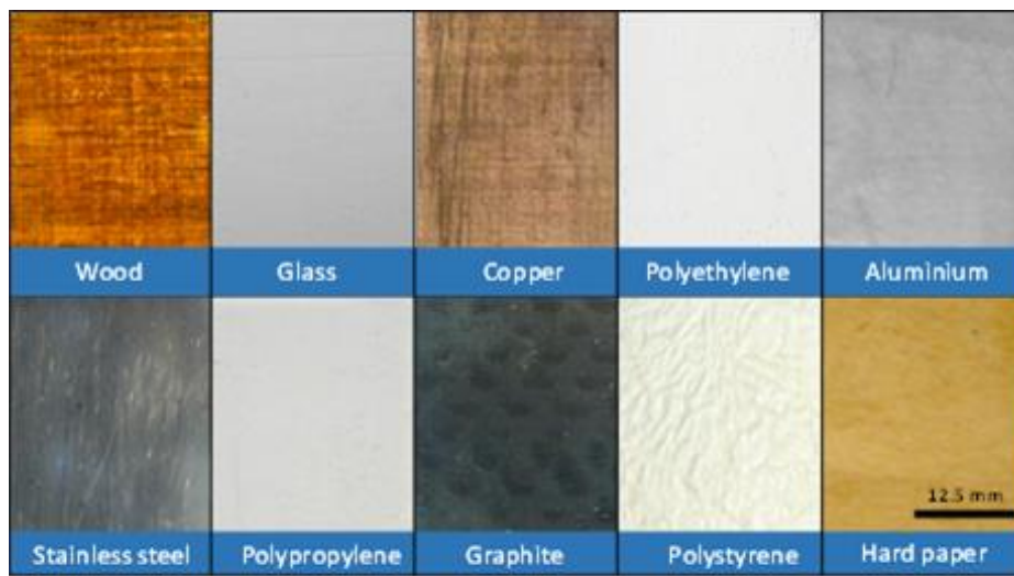
Figure 6.9 Universality of the coating. The coatings can be universally applied to all substrates from wood to plastic and the appearance of the substrate remains unchanged even after the coating. Reprinted with permission from publication III, (Baidya et al. , 2018) © 2018 John Wiley and Sons.
