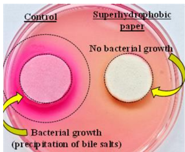
Figure 5.9 Demonstration of bacterial resistance property of superhydrophobic paper. This was compared with uncoated paper. Reprinted with permission from publication II, (Baidya et al. , 2018) © 2018 John Wiley and Sons.
