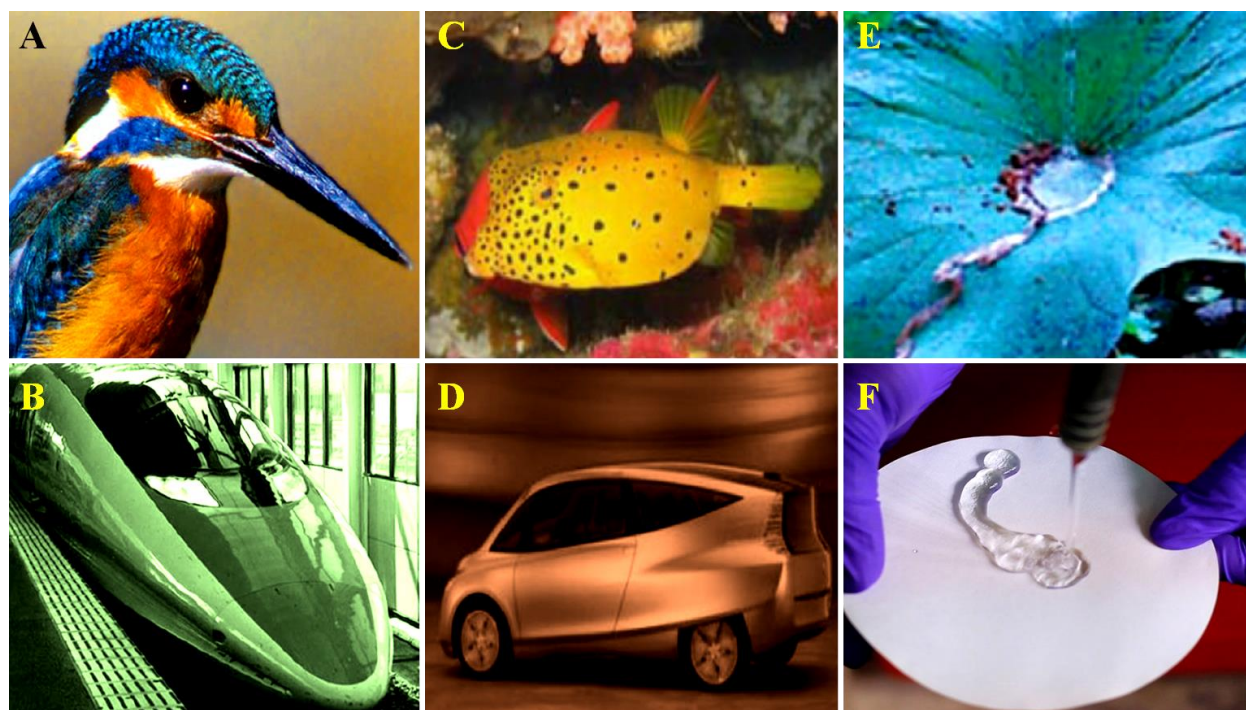
Figure 1.1 (A,B) Kingfisher's beak-inspired design of high speed train. Reproduced with permission from (Goel, 2013), © 2013 IEEE. (C,D) Box fish-inspired design of vehicle. Reprinted with permission from (Bannasch, 2009) © 2009 Springer
