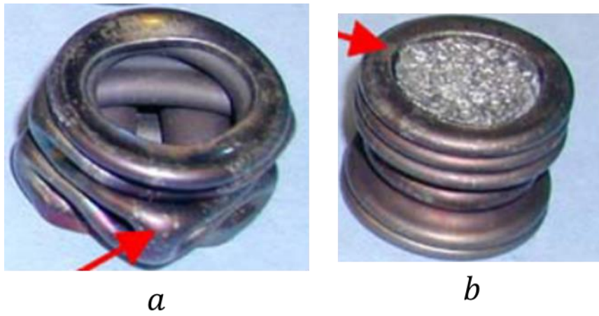
Figure 6: Diamond and concertina deformation modes of (a) empty- (b) foam-filled long tubes [57]
