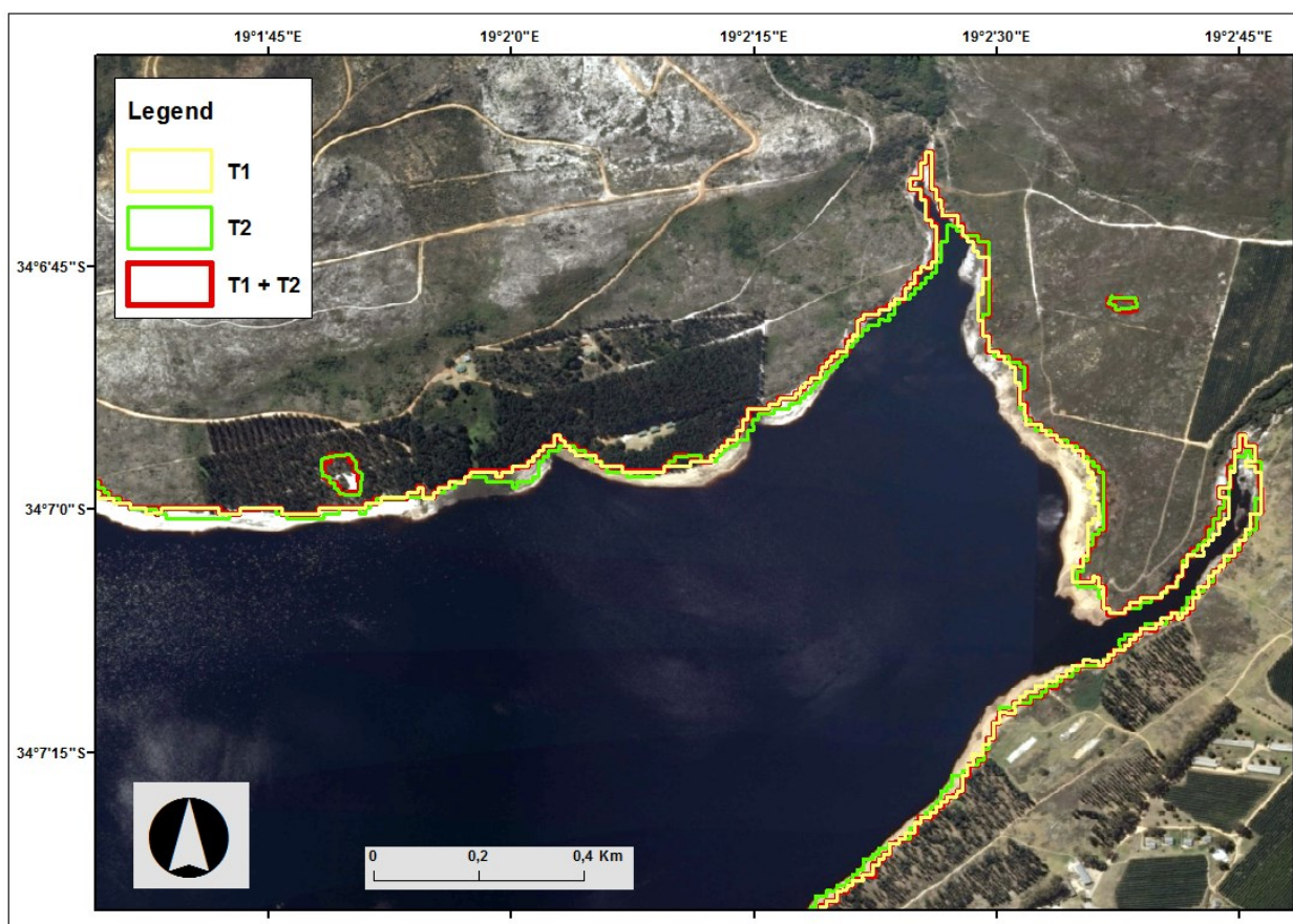
Figure 5.6 The visualisation of water masks derived from T1 (NDWI), T2 (SAR VH band) and T1+T2 (fusion of T1 and T2). An aerial photograph of October 2014 was used at which time the water level was lower than those at T1 and T2.
