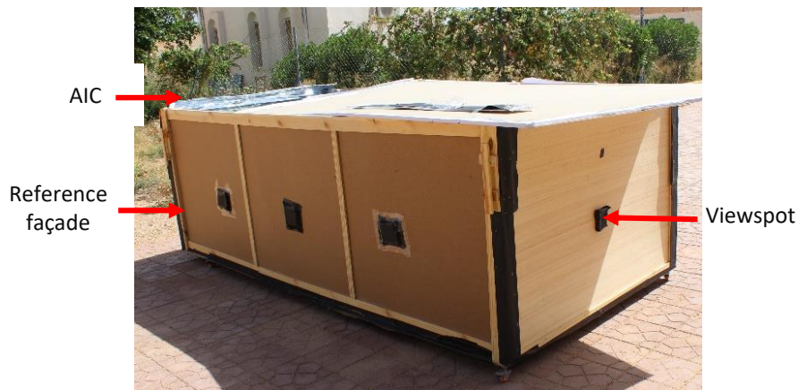
Figure 3. Physical scale model and Viewspot position
