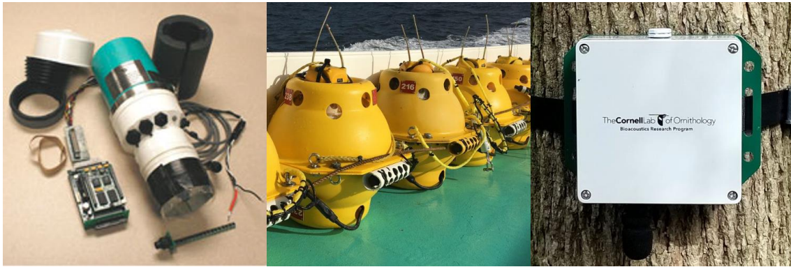
Figure 3. Left: disassembled ARU. Middle: MARUs in transit to a deployment location. Right: Swift unit strapped to a tree. (Bioacoustics Research Program)
