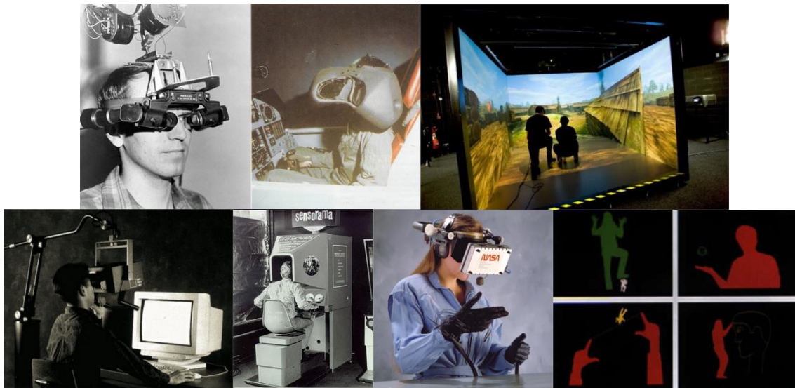
Figure 6. Top row (Left to right): The Sword of Damocles, VCASS, CAVE. Bottom row (Left to right): BOOM, Sensorama, VVED, Videoplacé.
