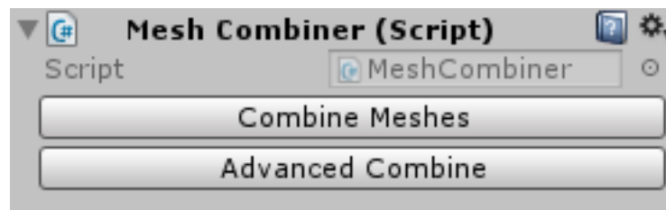
Figure 39. Part of the inspector window of an object with the Mesh Combiner editor script attached to it. If the script were left unaltered, this part of the inspector window would contain nothing but the name of the script. However, for the purpose of combining game object meshes in edit mode, the editor script was altered to add two functional buttons which, when clicked, combine the meshes of all the game object's children into a single mesh that is added to the game object.
