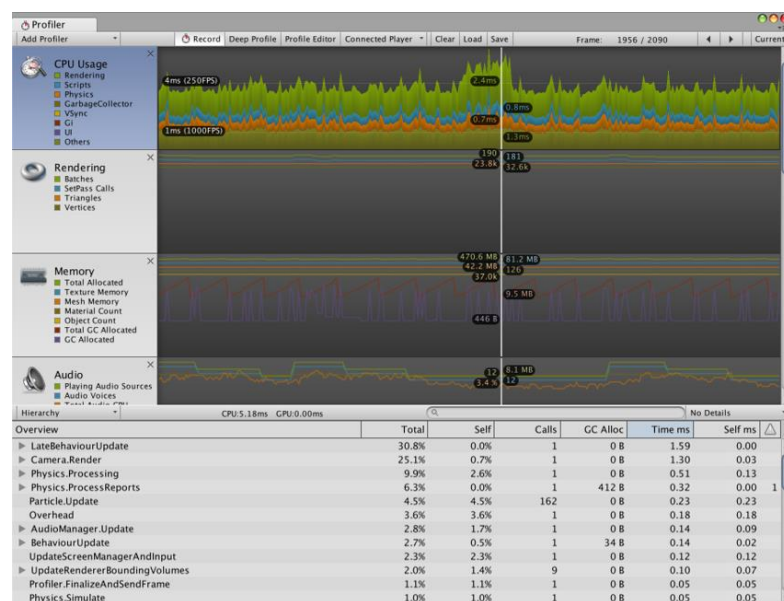
Figure 11. The profiler window. The window's upper section shows the resources (CPU, Rendering, etc.) being used by the game on a timeline containing a graph which shows data usage. The data at the bottom of the window correspond to a specific frame. The frame can be changed by moving the white vertical line across the timeline.
