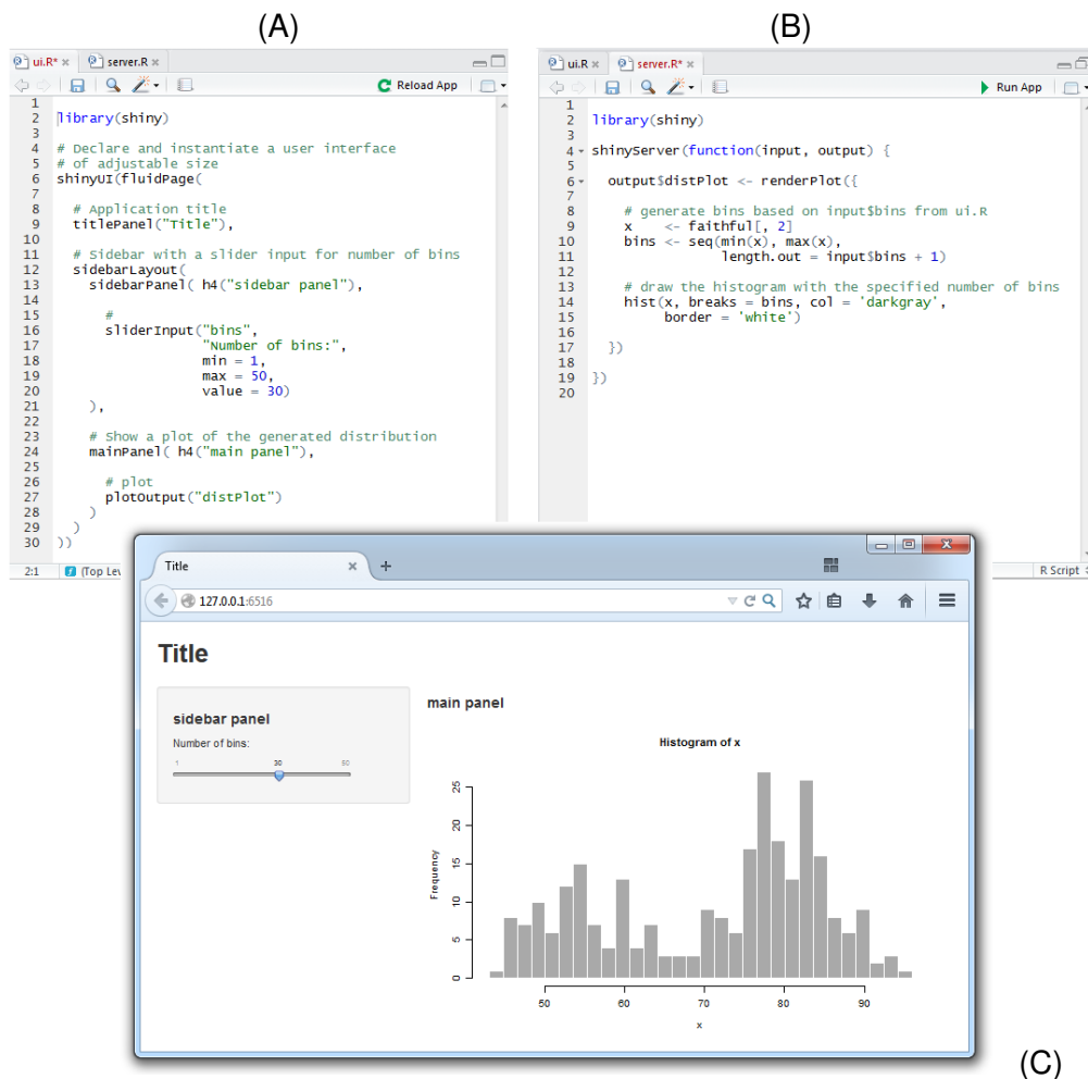
Figure 3.8: Basis structure of SHINY applications. This figure depicts the basic example from the RSTUDIO documentation of the SHINY package: a reactive histogram, whose bar size (number of bins) can be changed by a slider. [R114]. (A) The user-interface script ui.R describes the basic composition. (B) The server script server.R defines the underlying computations needed for reactivity. (C) Final reactive web application.
