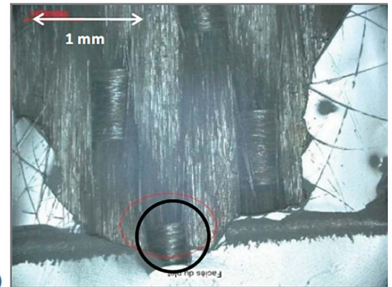
Fig. 4. (a) Fracture surfaces of treated substrates after the three-point bending test showing the two types of initiation, (a) adhesive and (b) cohesive. The location of the initiation is represented by the circles.
