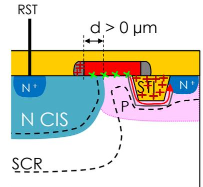
The overlap between the gate and the photodiode protect from TID induced defects in the spacer
