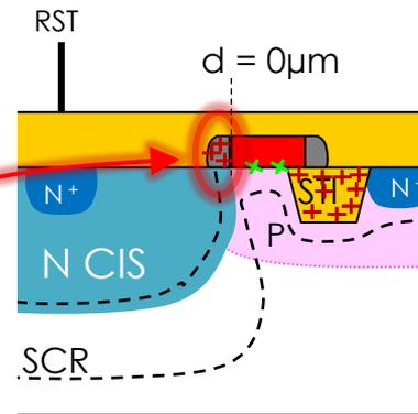
Induced defects in the spacer contribute to the dark current
