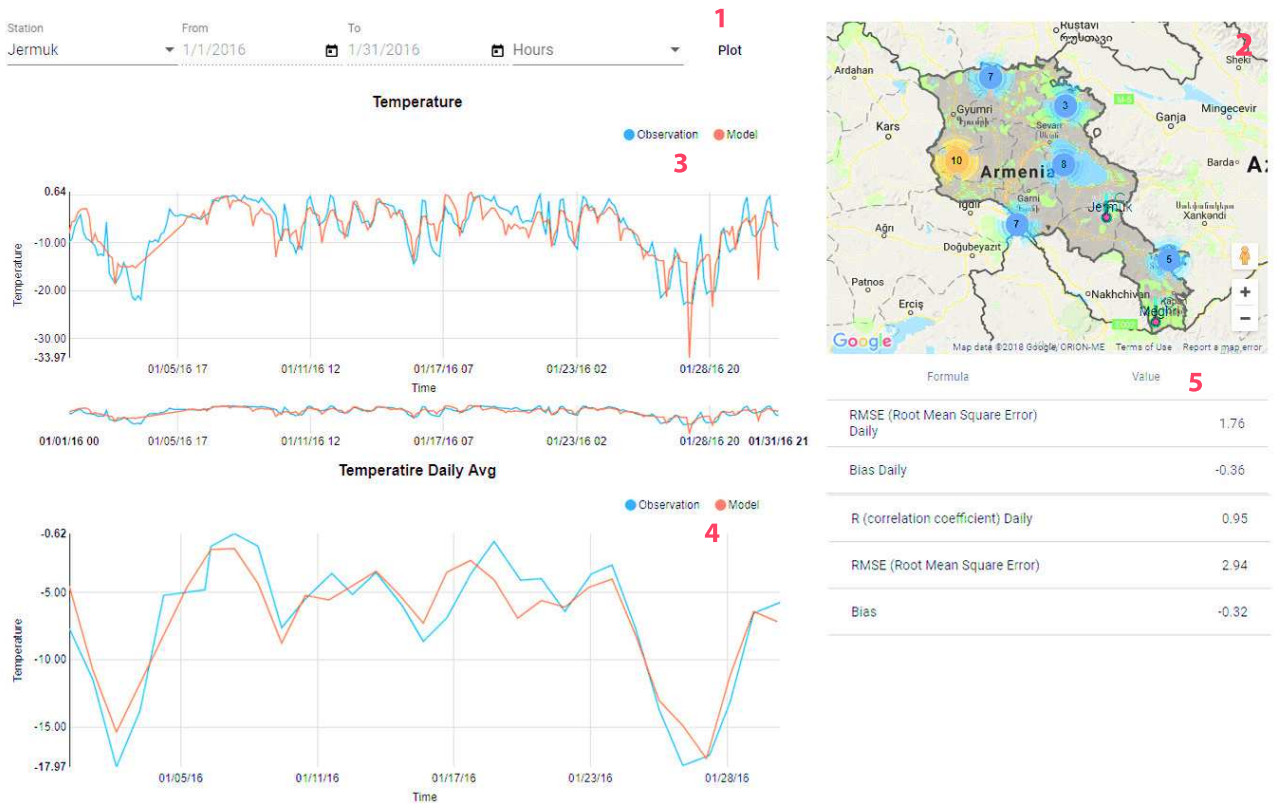
FIG. 2.3. Web-based visualization and analytical platform consists of the following sections: 1- query form, 2 - map, 3 - temperature chart, 4 - daily average temperature chart, 5 - coefficients table.
