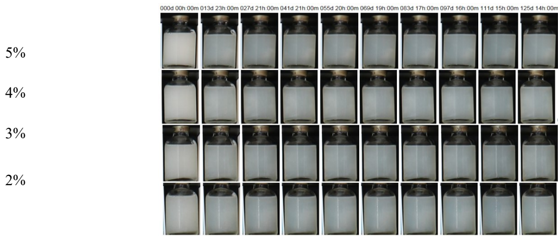
Figure 5.10: Loading test of the sample at HCO= [0.4%] with different aeration levels (ranging from 2 to 5%) at fixed Temperature (30°C)
