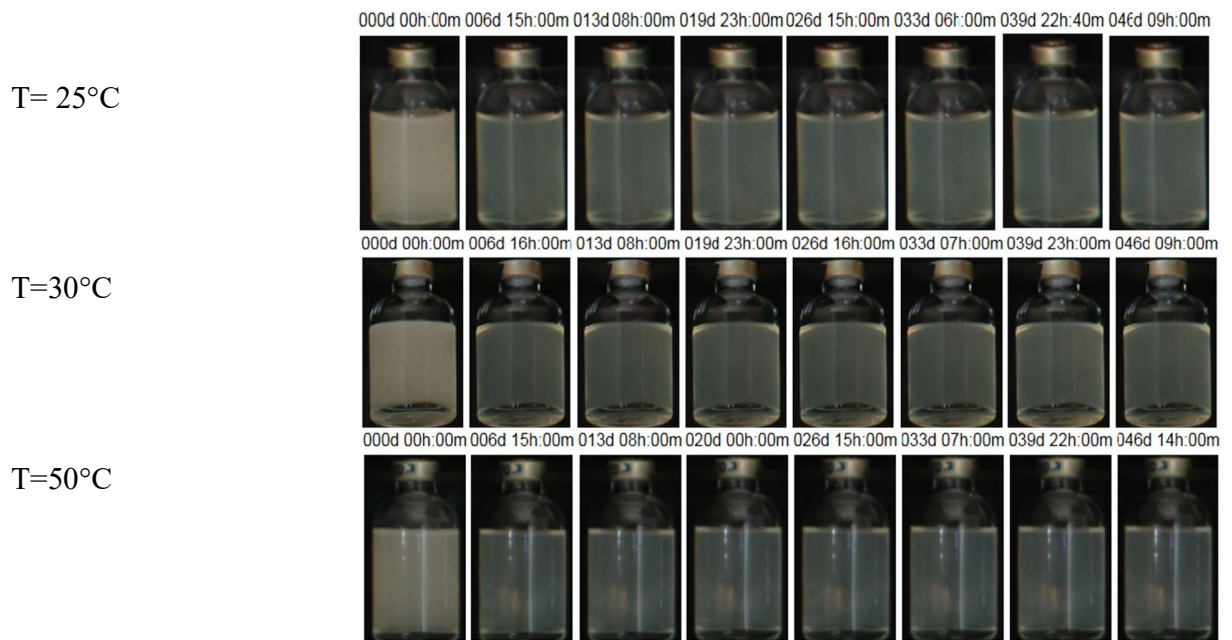
Figure 5.7: Time Evolution of Loading Test Samples at HCO = [0.1\%] at different temperatures with the initial air bubbles volume fraction equal to 3%.
