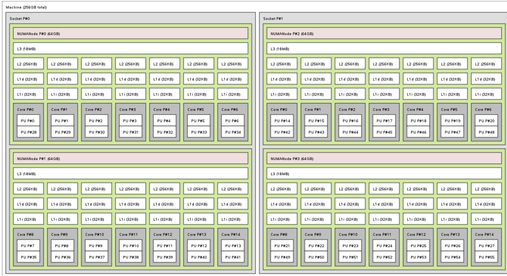
Figure 1.3: Topology of one Haswell node of SuperMUC Phase 2, taken from [65].
