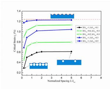
**Figure 4.2.3**. The strain for first bifurcation as a function of spacing *L* in the bilayer with cavities having different diameters and depths.
