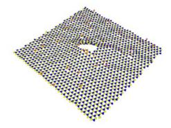
**Figure 2.1.S5.** The nucleation of pore on a single layer of boron nitride (BN) with a SiO2 NP supported (1 nm) at 170 ps. This is exemplified to show the applicability of strainguided perforation to a broad variety of 2D materials. Simulation parameters: temperature of 1600K, oxygen concentration of  $4 \times 10^{-3}$ /Å<sup>3</sup>.
