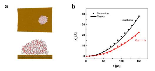
**Figure 2.2.5** (a) Top view and side view of 500-water-molecule droplet on copper (111) surface. (b) Comparison of displacement-time curves of 500-water-molecule droplet on graphene and copper (111) surface.
