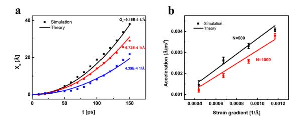
Figure 2.2.3 (a) The time history of the displacement of the mass center of the 500-watermolecule droplet for various strain gradient  $G_x$ . (b) The acceleration of the mass center of the droplet with respect to strain gradient  $G_x$  for various sizes of the droplet.
