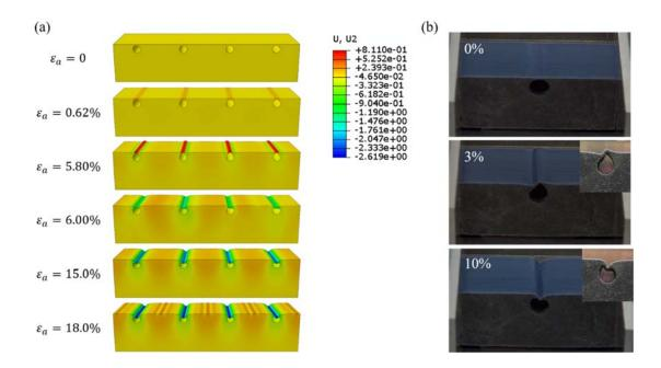
Figure 4.2.2. Simulation (a) and experiment (b) images of the defected bilayer structure at various compressive strains, where  $D/\lambda_{wc} = 1$ ,  $h/\lambda_{wc} = 0.1$  and  $L/\lambda_{wc} = 5$ .
