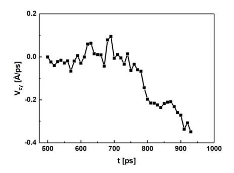
**Figure 2.2.S4.** The time history of velocity component in the *y* direction for water droplet on a monolayer graphene with tunable strain gradient direction.
