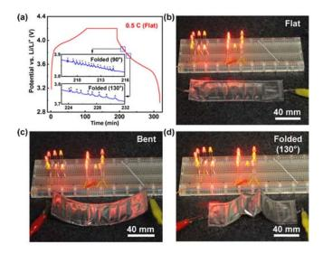
**Figure 5.2.5** a) Voltage profile for the foldable battery under continuously and manually 90° and 180° folding during discharge. b-d) Practical applications of foldable battery to power a series of LEDs in flat, bent and folded configurations.
