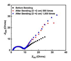
**Figure 5.2.S2. Electrochemical Impedance Spectroscopy (EIS) of the foldable battery in the flat state before and after bending 500 and 1,000 times, respectively.** The frequency of EIS test is from 1MHz to 0.1 Hz. The data shows that even after bending 1,000 times with a diameter of 2 cm, the charge transfer resistance changed little, which indicates that our battery is mechanically robust.
