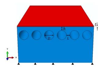
**Figure 4.2.1**. A representative segment of thin film (red) adhered to defected substrate (blue) with pre-patterned holes.
