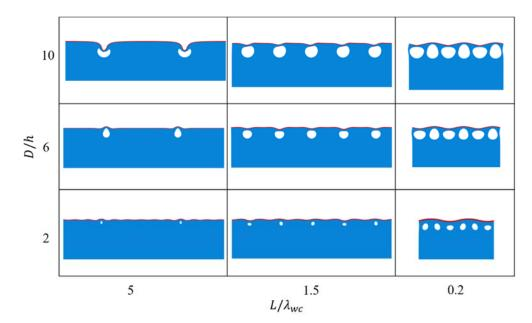
Figure 4.2.5. The diagram of surface morphologies for the defected structures  $(h/\lambda_{wc} = 0.1)$ , where the applied strain is fixed at  $\varepsilon_a = 0.02$ , against normalized diameter D/h and normalized spacing  $L/\lambda_{wc}$
