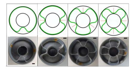
**Figure 7.1.2** The morphologies of elastic rings confined in annular solid constraints. Except the single-blister one, external displacements have to be applied as initiators to overcome energy barrier of forming higher-order buckling morphologies.
