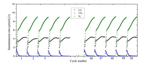
Figure 5.1.S12. The cyclic elution profiles for  $La_{0.95}Cu_{0.05}FeO_{3-\delta}$  in the POx step over 50 cycles.
