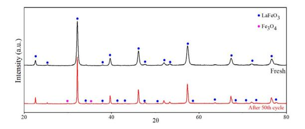
Figure 5.1.S14. The XRD patterns for the as-prepared and the re-oxidized  $La_{0.95}Cu_{0.05}FeO_{3-\delta}$  sample after 50 cycles.
