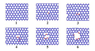
**Figure 2.1.S2**. The simulated perforation process on graphene by oxygen at the atmosphere with the oxygen number density  $4 \times 10^{-3}$ /Å<sup>3</sup> and the temperature 1300 K: 1) bare graphene (0 ps); 2) oxygen adsorption (70 ps); 3) lattice distortion (105 ps); 4) bond breaking (125 ps); 5) single vacancies (150 ps); 6) pore growth (165 ps). In this simulation, the diameter of NP underneath is 1 nm.
