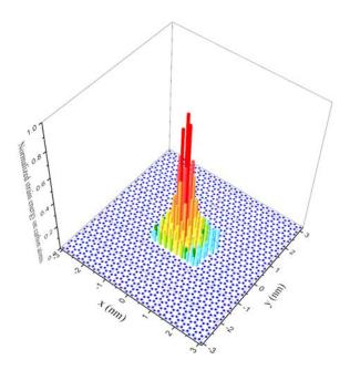
**Figure 2.1.S8**. Spatially discrete distributions of normalized strain energy  $\varepsilon$  on each carbon atoms calculated by SFN model.
