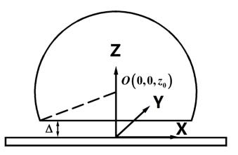
Figure 2.2.S2. Sketch of a spherical-cap drop in the coordinate system.
