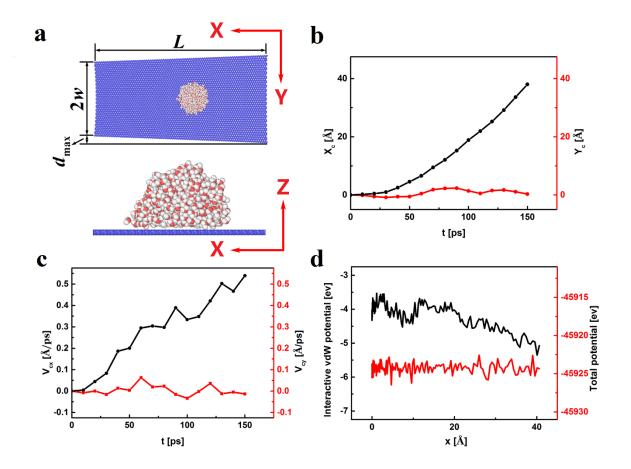
**Figure 2.2.2** (a) Top view and side view of a 500-water-molecule droplet on a monolayer graphene. (b) The time history of the displacement of the mass center of droplet along the x direction. (c) The time history of the velocity of the mass center of droplet along the x direction and y direction. (d) The <u>variation</u> of interactive vdW potential energy and the system total potential energy with respect to the transport distance x.
