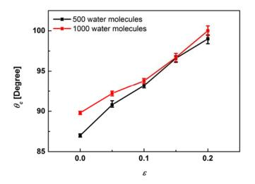
Figure 2.2.S1. Variation of the contact angle with the strain  $\varepsilon$  and size of the droplet.
