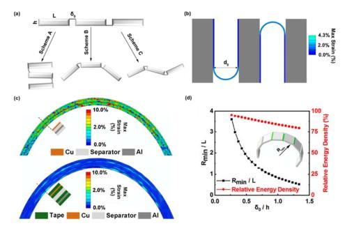
Figure 5.2.2 Structural design for the zigzag foldable battery.
