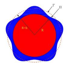
**Figure 3.1.1**. The schematic of a spherical core/shell structure: the radius of core is denoted by *R* and the shell have thickness *h*.
