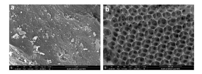
Figure 5.1.S4. SEM images of the (a) conventional and (b) macroporous  $La_{0.95}Cu_{0.05}FeO_{3-\delta}$  samples. The macroporous  $La_{0.95}Cu_{0.05}FeO_3$  exhibited a well-defined three-dimensional periodic framework with the pore diameter of  $100 \pm 10$  nm.
