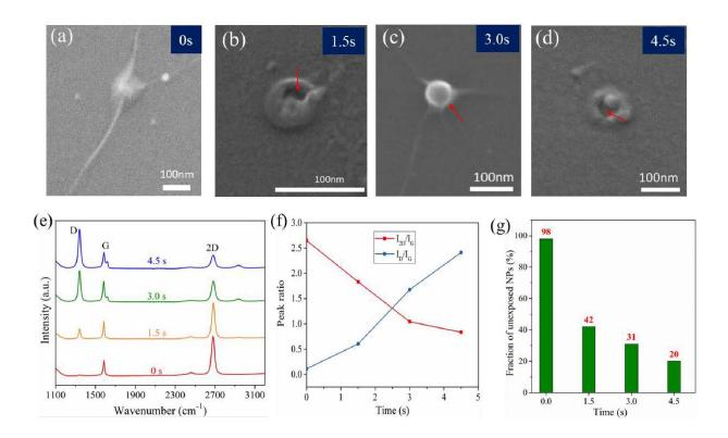
**Figure 2.1.5 The effect of exposure time on pore growth.** Time evolution of (a)-(d) SEM images of created pores. (e) Raman spectra of graphene with increasing exposure durations to oxygen plasma; (f) The ratio of  $I_D/I_G$  and  $I_{2D}/I_G$  for etching graphene undergoing different exposure times; (g) Statistical summary on the number ratio of unexposed NPs to total sampling NPs as a function of different exposure time.
