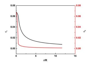
**Figure 2.1.S7**. Continuous distributions of radial strain  $\varepsilon_r$  and tangential strain  $\varepsilon_{\theta}$  as a function of the horizontal distance away from the NP's center, which is calculated by SBA model.
