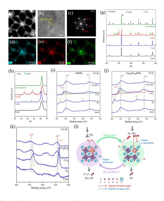
Figure 5.1.3 Structural and compositional characterizations for fresh and spent La<sub>0.95</sub>Cu<sub>0.05</sub>FeO<sub>3-δ</sub>. (a) STEM image, (b) HRTEM image, (c) the corresponding Fast Fourier Transform image, (d-f) EDS maps for as-prepared La<sub>0.95</sub>Cu<sub>0.05</sub>FeO<sub>3-δ</sub> sample. (g)
