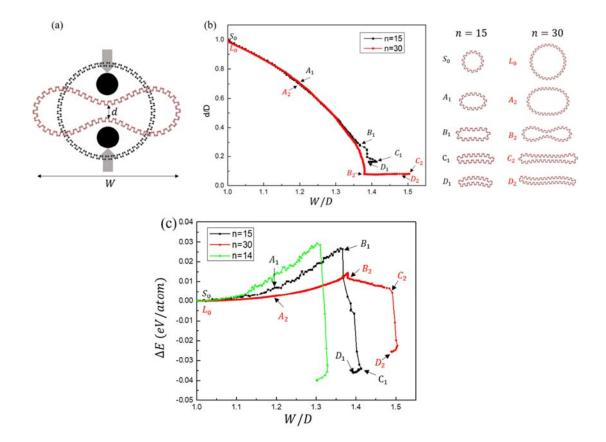
**Figure 2.4.1** (a) The schematic of deforming armchair PNT; (b) The deformation pathways of (0,15) and (0,30) armchair PNTs (left) projected to the d - W plane; (c) The strain energy  $\Delta E$  along deformation pathway as a function of W.
