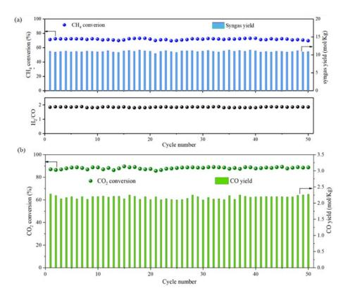
Figure 5.1.5. Redox stability of La<sub>0.95</sub>Cu<sub>0.05</sub>FeO<sub>3</sub> over 50 cycles. (a) Methane conversion, syngas yield and H<sub>2</sub>/CO molar ratio in the step of methane POx. (b) CO2 conversion and CO yield in the step of O<sub>2</sub>-containing CO<sub>2</sub> (CO<sub>2</sub>:O<sub>2</sub>=5:1) splitting.
