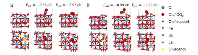
**Figure 51.S11**. (a) Side views and top views of the reduced LaFeO<sub>3</sub>(110) surface (left) and its  $CO_2$  (middle) and  $O_2$  (right) adsorption configurations. (b) Side views and top views of the Cu atom supported by reduced LaFeO<sub>3</sub>(110) surface (left) and its  $CO_2$  (middle) and  $O_2$  (right) adsorption configurations.
