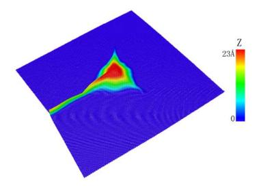
Figure 2.1.S11. Simulated wrinkling features surrounding bulges in r-MD simulations.
