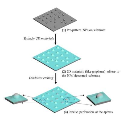
**Figure 2.1.1** Schematic of strain-guided perforation on 2D materials through pre-patterned NPs underneath
