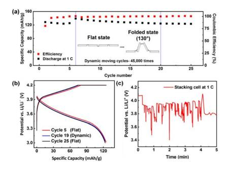
**Figure 5.2.4** Dynamic loading test of the foldable battery at 1 C. a) Cycling performance of a zigzag-like foldable battery in different states under dynamic and repetitive fold loading test. The inset shows the schematic of the flat and folding configurations. b) Galvanostatic charge-discharge voltage profiles for 5th, 19th, and 25th cycle. c) The discharge profile of a normal stacking cell at 1 C, subjected to lower folding frequency.
