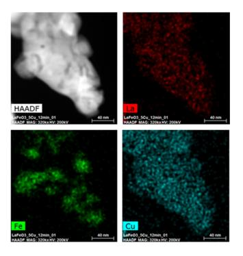
Figure 5.1.S7. STEM and EDS mapping images of deeply reduced La<sub>0.95</sub>Cu<sub>0.05</sub>FeO<sub>3-δ</sub> sample.
