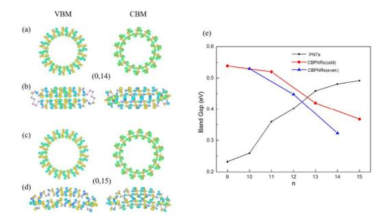
Figure 2.4.4 The spatial charge density associated with the VBM and CBM for the (a, c) PNTs and (c, d) CBPNRs for the size (0,14) and (0,15). The isosurface is set to 0.008  $e/b_0^3$ , and  $b_0$  is the lattice parameter along nanotube axis. (e)The band gaps of armchair PNTs and CBPNRs are plotted as a function of tube size n.
