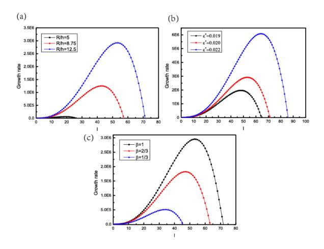
**Figure 3.1.2** The dimensionless growth rate plots as a function of various fluctuation mode degree *l* characterizing the evolved morphology at various values of (a) normalized size R/h, (b) intrinsic strain  $\varepsilon^*$  and (c) modulus ratio  $\beta$
