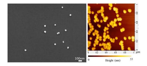
Figure 2.1.S10. SEM and AFM images of  $SiO_2$  NPs on  $SiO_2$  substrate, showing the diameter of NPs is roughly 50 nm
