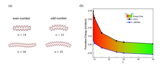
Figure 2.4.2 (a) The CBPNR configurations derived from the PNTs with odd or even value of n.; (b) The formation energy of PNTs and CBPNRs relative to that of monolayer phosphorene is dependent on the size n.
