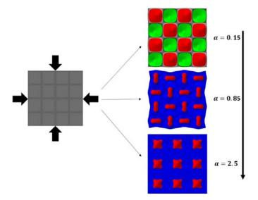
Figure 4.1.5 The surface morphologies of cuboidal cavity embedded CESMs with  $\alpha$  undergoing the same biaxial global compression of 12%.
