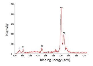
Figure 3.1.S1. EDS spectra obtained at the red dash region (in Figure 5(c)) by X-ray
