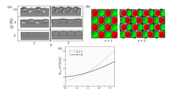
**Figure 4.1.4** (a) The phase diagram of simulated surface textures and (b) the surface morphologies of cuboidal cavity embedded CESMs for  $\gamma = 1$  and  $\gamma = 2$  at the uniaxial global compression of 14%. (c) Theoretically critical membrane forces of plates for different buckling modes *m* as a function of the aspect ratio  $\gamma$ .
