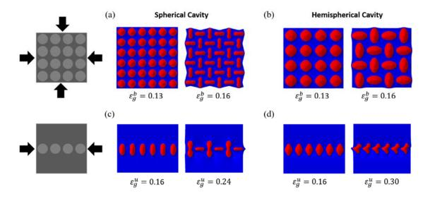
**Figure 4.1.6** The surface morphologies of CESMs with square patterns of (a) spherical and (b) hemispherical cavities undergoing different biaxial global compression. The surface morphologies of CESMs with one column of (c) spherical and (d) hemispherical cavities undergoing different uniaxial global compression.
