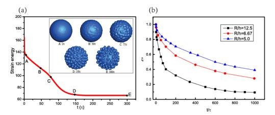
Figure 3.1.3 (a) The evolution of strain energy of the spherical core/shell particle ( $R = 50l, h = 4l, \beta = 1/3$ ) as a function of dimensionless time. (b) The coverage parameter  $\xi$  as a function of simulation time for three cases: R/h = 12.5; R/h = 6.67; R/h = 5.0.
