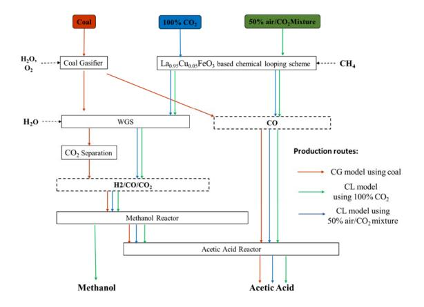
Figure 5.1.S15. Diagram of routes for synthesizing methanol and acetic acid using CG and CL models.
