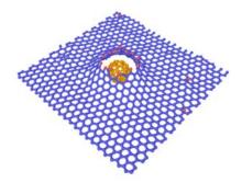
Figure 2.1.86. Perforation of graphene with NPs of chemically stable C60 fullerence. Simulation parameters: NPs' size (7Å), snapshot time (220ps), temperature (1600K), oxygen concentration  $(4 \times 10^{-3} / \text{Å}^3)$ .
