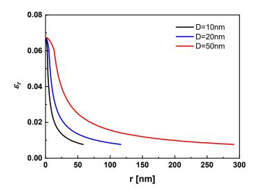
Figure 2.1.89. Continuous distributions of radial strain  $\varepsilon_r$  for the NPs with different size, which calculated by SBA model. This result verifies the independence of maximum strain at the dome apex on the size of NP.
