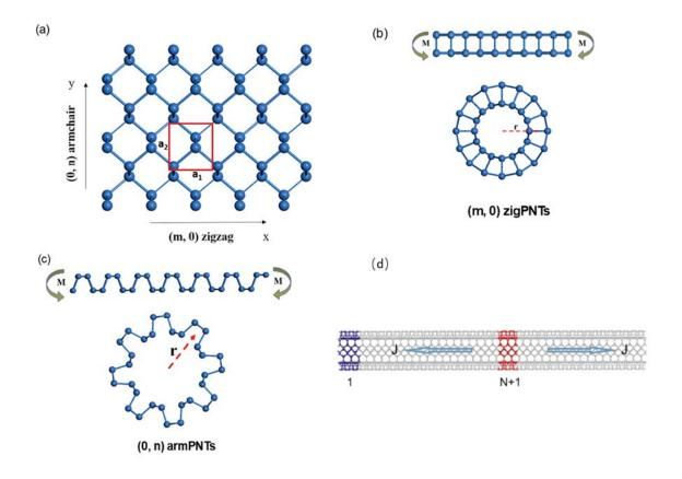
**Figure 2.3.1** (a) Top view: crystal structure of 2D phosphorene ( $a_1 = 3.3$  Å and  $a_2 = 4.5$  Å); (b) The zigPNT is bended from phosphorene sheet along the wrapping vector (m, 0) ( $r = ma_1/2\pi$ ); (c) the armPNT is bended from MBP along the wrapping vector ( $r = a_2/2\pi$ ); (d) An arm-PNT is divided into 2N layers, with the cold layer 1 and hot layer N+1.
