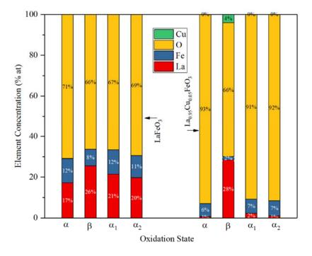
**Figure 5.1.S8.** Surface elemental composition (XPS data) of LaFeO<sub>3</sub> and La<sub>0.95</sub>Cu<sub>0.05</sub>FeO<sub>3- $\delta$ </sub> samples under different oxidation states: as-prepared (label:  $\alpha$ ), reduced by H<sub>2</sub> (label:  $\beta$ ), re-oxidized by CO<sub>2</sub> (label:  $\alpha_1$ ) and re-oxidized by O<sub>2</sub>-containing CO<sub>2</sub> (label:  $\alpha_2$ ).
