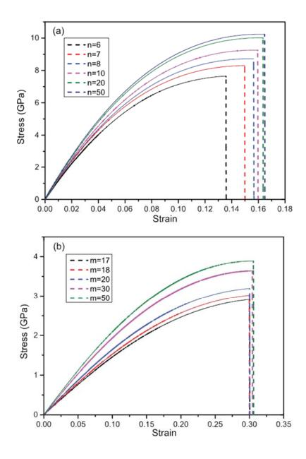
Figure 2.3.3 The axial tensile stress-strain curves for (a) armPNTs and (b) zigPNTs with various wrapping indexes at T = 0 K
