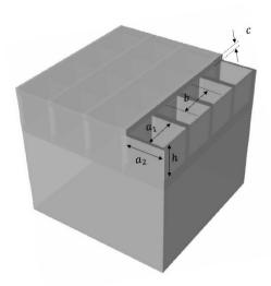
Figure 4.1.3. Schematics of representative CESMs with patterned cuboidal cavities.
