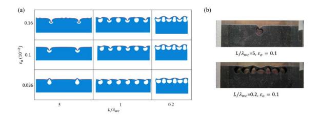
Figure 4.2.4. The diagram of buckling morphologies for the defected structures  $(D/\lambda_{wc} = 1 \text{ and } h/\lambda_{wc} = 0.1)$  against applied strain and normalized spacing.
