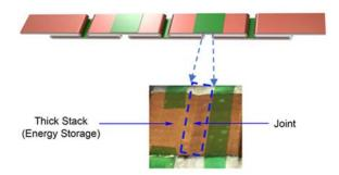
Figure 4.3.83. The magnified optical image to illustrate the folding joint.
