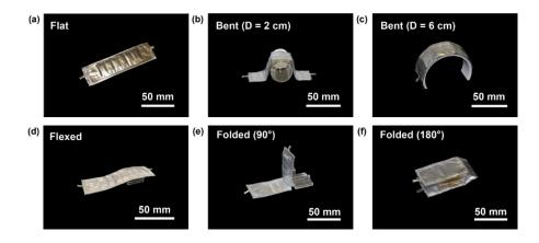
Figure 5.2.S1 Different states of the foldable battery during long cycle performance in Figure
