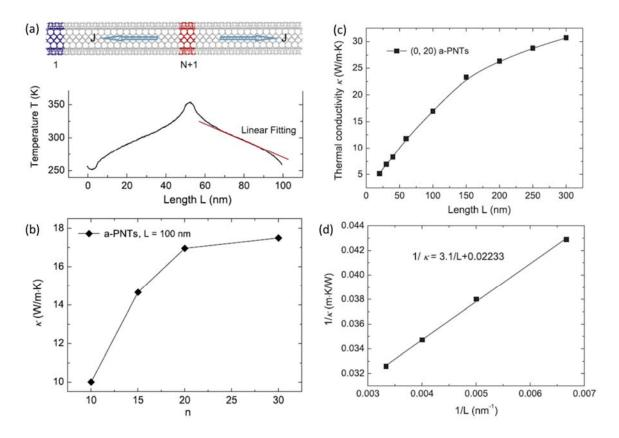
**Figure 2.3.6** (a) An arm-PNT is divided into 2*N* layers, with the cold layer 1 and hot layer N + 1; (b) The diameter-dependent thermal conductivity of arm-PNT; (c) The thermal conductivity  $\kappa$  of arm-PNT with varying axial length under temperature T = 300 K; (d) Linear fitting of the relationship between the inverse of  $\kappa$  and the inverse of *L*.
