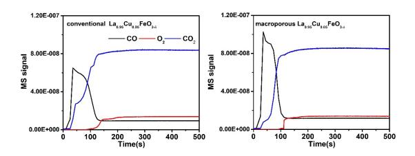
**Figure 5.1.S5.** The oxidation of reduced conventional and macroporous  $La_{0.95}Cu_{0.05}FeO_{3-\delta}$  samples by the O<sub>2</sub>-containing CO<sub>2</sub>.
