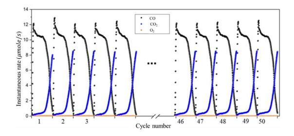
**Figure 5.1.S13.** The cyclic elution profiles for  $La_{0.95}Cu_{0.05}FeO_{3-\delta}$  in the step of O<sub>2</sub>-containing CO<sub>2</sub> (CO<sub>2</sub>: O<sub>2</sub> = 5:1) splitting over 50 cycles.
