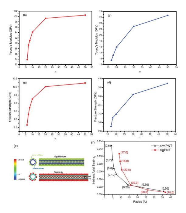
**Figure 2.3.4** Size-dependent mechanical properties at T = 0 K. Young's modulus of (a) armPNTs and (b) zigPNTs, fracture strength of (c) armPNTs and (d) zigPNTs. (e) The atomic stress (unit: eV/atomic volume) of PNT structures. (f) The intrinsic axial strain in each sublayer of equilibrium armPNTs (black line) and zigPNTs (red line) at T = 0 K.
