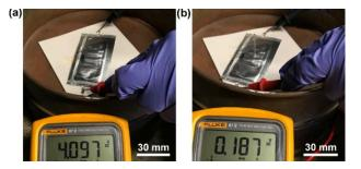
**Figure 5.2.S5.** The flammable test of the foldable battery. After fully charge at 0.5 C, the voltage image of the foldable battery a) before punctuation and b) after punctuation. The result shows that battery was still in stable condition after punctuation without catching smoke or fire.
