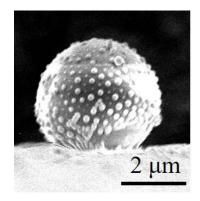
**Figure 3.1.S2**. The Ag core/SiO<sub>2</sub> shell microstructures (approximate radius of 2.5  $\mu$ m) shows a non-uniform pattern of islands and the annealing time is 5 min.
