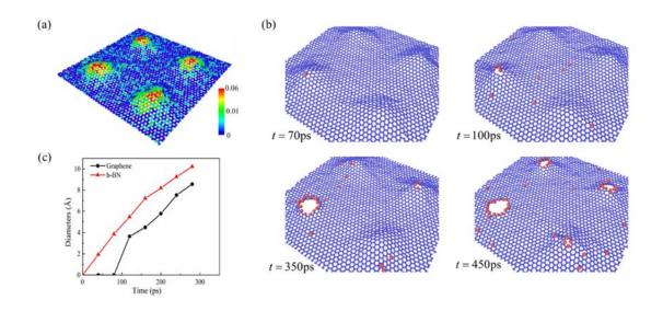
**Figure 2.1.2 r-MD simulations demonstration.** (a) Strain distribution of graphene adhered to the substrate decorated with NPs array having diameter of 1 nm and periodicity of 5 nm; (b) The morphological evolution of etched graphene with respective to simulation time; (c) The area of created pores as a function of simulation time for graphene and h-BN.
