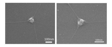
**Figure 2.1.S12**. SEM images of initiated perforation at wrinkling ridges of graphene after exposure to oxygen plasma for 1.5 s
