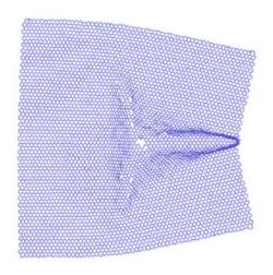
Figure 2.1.S13. r-MD simulation result of initiated perforation at wrinkling ridges. Simulation parameters: NPs' size (2 nm), snapshot time (65 ps), temperature (1600K), oxygen concentration  $(3 \times 10^{-3} / \text{Å}^3)$ .
