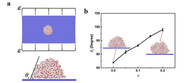
Figure 2.2.1. (a)Top view and side view of a 500-water-molecule droplet on a monolayer graphene with a constant uniaxial strain  $\varepsilon$ . (b) Variation of the contact angle with the strain  $\varepsilon$ .
