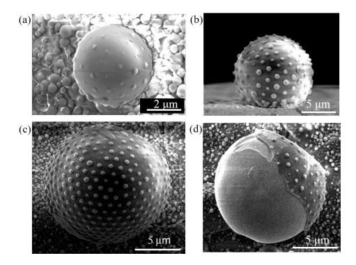
**Figure 3.1.6** SEM micrographs of the Ag core/SiO<sub>2</sub> shell microstructures annealed for 10 min, with approximate radii (a) 2.5  $\mu$ m, (b) 4.0  $\mu$ m and (c) 7.5  $\mu$ m. A broken sample with smooth Ag core partially covered by SiO<sub>2</sub> shell is shown in (d) under a cooling rate of 500 K/min.
