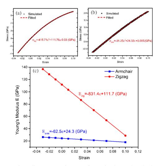
Figure 2.3.5 The nonlinear stress-strain curves of a 2D phosphorene sheet simulated by MD at T = 0 K along the (a) zigzag direction and (b) armchair direction; The Young's moduli of the phosphorene sheet along zigzag direction (red line) and armchair direction (blue line) are fitted and plotted as a function of the applied strain, in (c).
