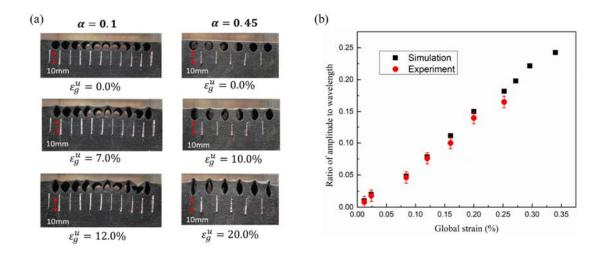
Figure 4.1.2 (a) Experimental surface evolutions of 3D-printed CESM prototypes with different values of  $\alpha$ , while  $\beta$  is set to be 0.2. (b) The comparison of amplitude-wavelength ratio between the simulation and experiment for  $\alpha = 0.45$
