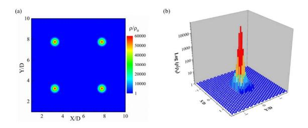
**Figure 2.1.3 Mechanism clarification.** (a) Spatially continuous distribution of perforation probability by SBA model; (b) Spatially discrete distribution of perforation probability by SFN model, where a single NPs is covered by graphene with periodic boundary condition.
