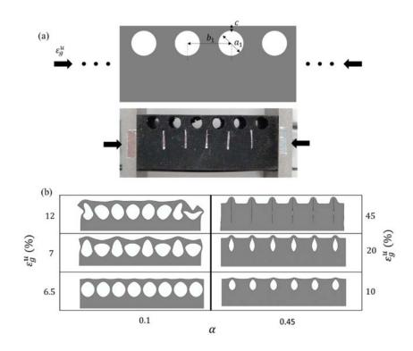
**Figure 4.1.1** (a) The top figure: a representative segment of a CESM under a global compressive strain and with labeled geometrical dimensions; the bottom figure: the experimental setup of uniaxial compressing the 3D printed material. (b) The phase diagram of simulated surface textures with respective to the uniaxial compressive strain.
