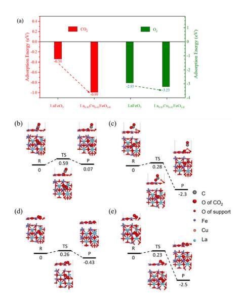
**Figure 5.1.4 DFT simulation results.** (a) Comparison of adsorption energies for CO<sub>2</sub> and O<sub>2</sub> on the (110) surfaces of reduced LaFeO<sub>3</sub> with and without Cu adatom; Reaction pathways of CO<sub>2</sub> splitting into oxygen atom and monoxide molecule on (b) the reduced LaFeO<sub>3</sub> (110) surface and (c) the reduced LaFeO<sub>3</sub> (110) surface with Cu adatom; Reaction
