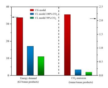
**Figure 5.1.6. ASPEN simulation results.** Comparison of (a) energy demand and (b) CO<sub>2</sub> emission for generating one metric ton of methanol and acetic acid as valuable products among three main models: the state-of-art coal gasification model, the chemical looping model using 50% CO<sub>2</sub> mixture and using 100% CO<sub>2</sub>.
