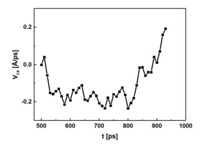
**Figure 2.2.S3** The time history of velocity component in the *x* direction for water droplet on a monolayer graphene with tunable strain gradient direction.
