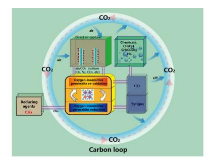
**Figure 5.1.1. Schematic of cyclic redox scheme and its contribution to close the carbon looping.** Three key processes are included: upstream direct-air-capture for producing aircontaining CO<sub>2</sub>, perovskites-based chemical looping reactor for syngas and CO production, downstream utilization of CO/syngas and subsequent CO<sub>2</sub> emission.
