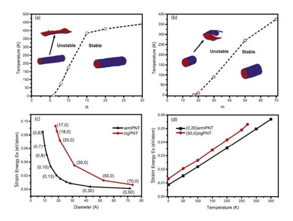
**Figure 2.3.2** The phase diagrams for thermal-stability of (a) armPNTs and (b) zigzagPNTs with varying temperature and wrapping vector of nanotube; (c) The strain energy stored in wrapped PNTs as function of the diameter of armPNTs (black triangular) and zigPNTs (red
