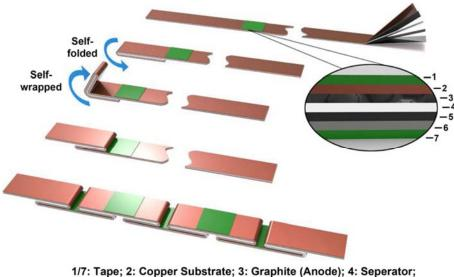
5: Lithium cobalt oxide (Cathode); 6: Aluminum Substrate.
