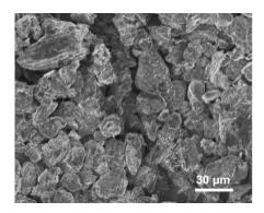
Figure 5.2.S4. The SEM image of anode at the joint with 2,000 more folding cycles than that
