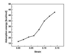
**Figure 2.1.S4.** Oxygen adsorption energy as a function of strain on graphene. The adsorption energy increases significantly with increasing bend-induced strain.
