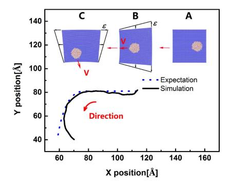
**Figure 2.2.4** Trajectory of water droplet on a monolayer graphene with tunable strain gradient direction.
