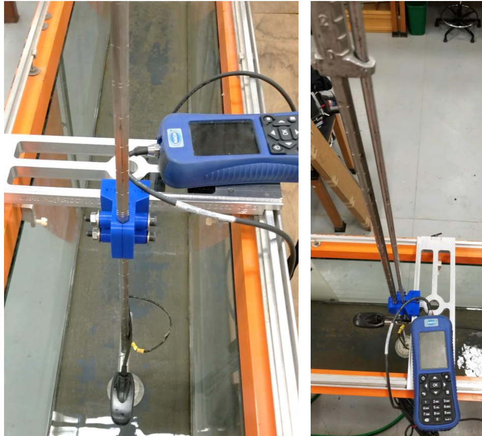
Figure 19: Hach Meter Testing Set Up for Fluid Velocity Characterization
