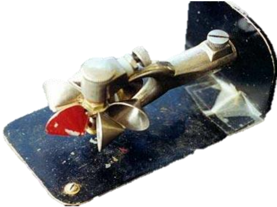
Figure 7: Pigmy Current Meter Example (Humboldt)
