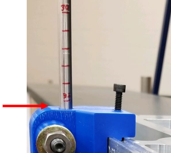
Figure 14: Pitot Tube Scale Positioning with Device 36 Centimeters Above Floor
