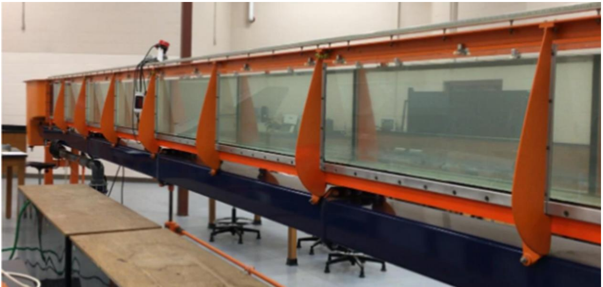
Figure 3: Armfield Experimental Tilting Glass Flume at Central State University (Sherping, 2019)
