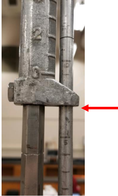
Figure 13: Wading Pole Scale Positioning with Sensor 2.5 cm Above Floor
