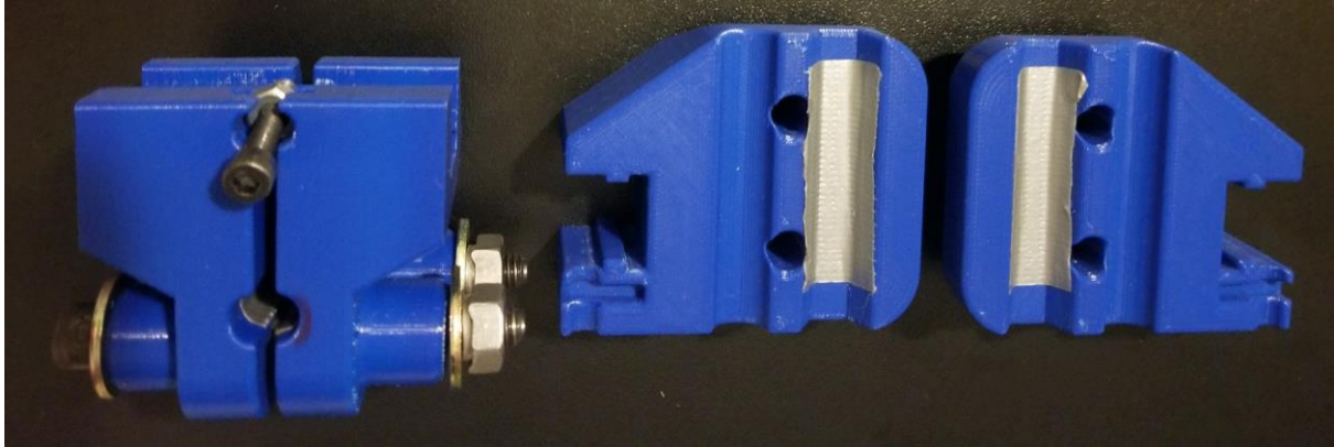
Figure 15: Wading Pole and Pitot Tube Mounts for Traverse System
