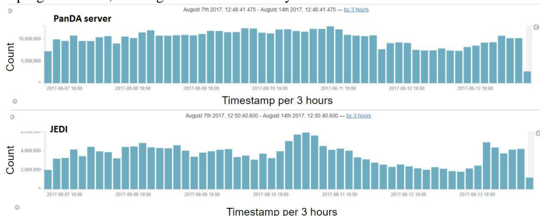
Figure 3. Graphics taken from Kibana with the number of entries received from Logstash, in the period from August 7 to August 14, with 3 hours interval.
