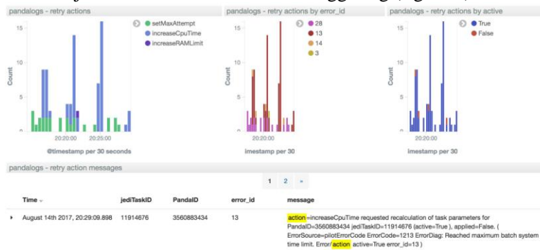
Figure 6. A snapshot of the retry module dashboard. From left to right, the plots show the incident breakdown by action, rule and whether the rule is active/passive. Messages/plots can be filtered for a given task or job ID for easy debugging.
