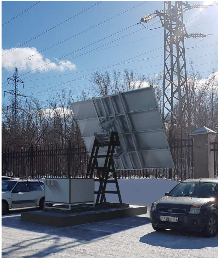
Figure 5. The sunny panel with the tracker system (development of Tomsk polytechnic university).
