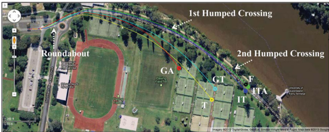
Fig. 11. Trajectories generated with KLT Techniques combined with double dogleg optimization method at 10 Hz, circle represent the end of each trajectory: green ITA; blue IT; cyan GT; yellow T; red GA; black F ground truth reference for final position (defined in Section 5.3 and Fig. 12).
