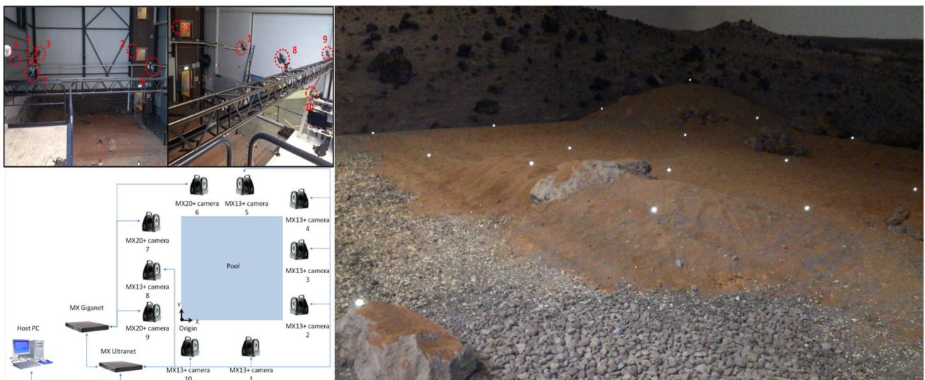
Fig. 6 Top left two views of the final cameras position; bottom left final Vicon architecture; and right ESA’s laboratory pool reproducing a Mars ground-like environment
