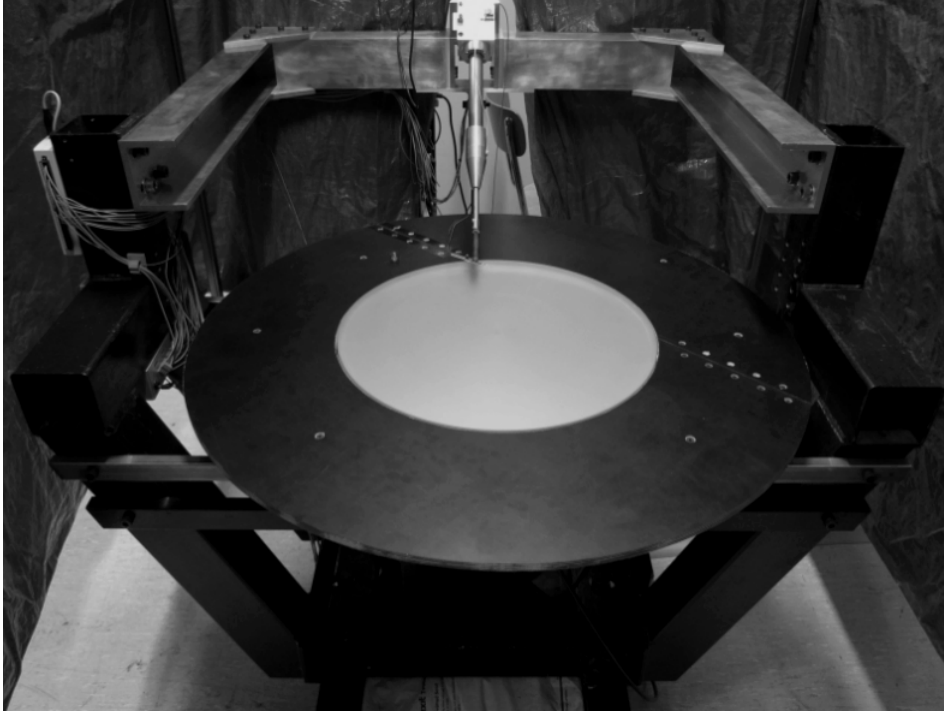
Figure 2.1: Rotating disk experimental arrangement by Imayama (2012), showing float glass disk and concentric annulus.
