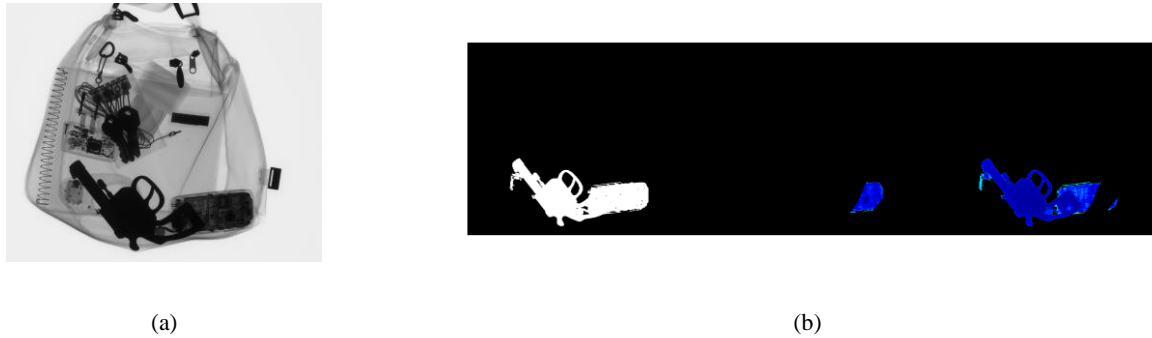
Figure 7. (a) Single-energy X-ray imagery of a bag (b) weapon cluster disjoint (X-ray image from 18 )
