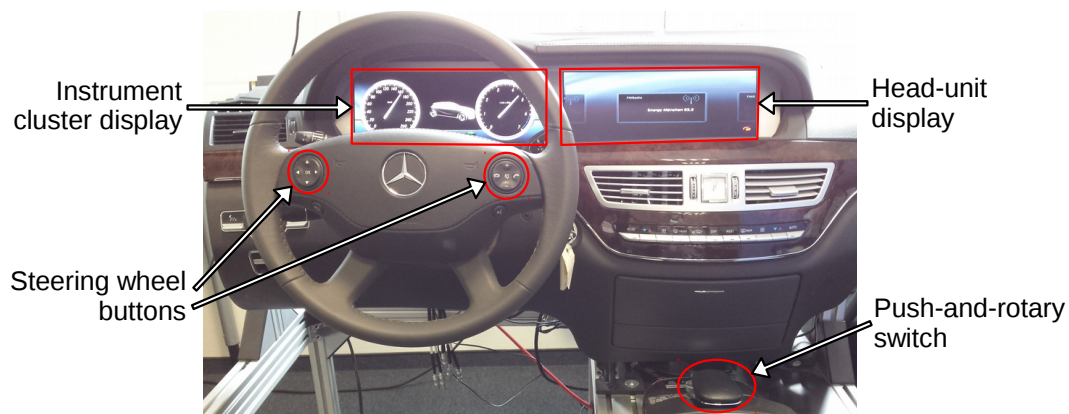
Figure 2.2.: Demonstrator front view with HMI devices
