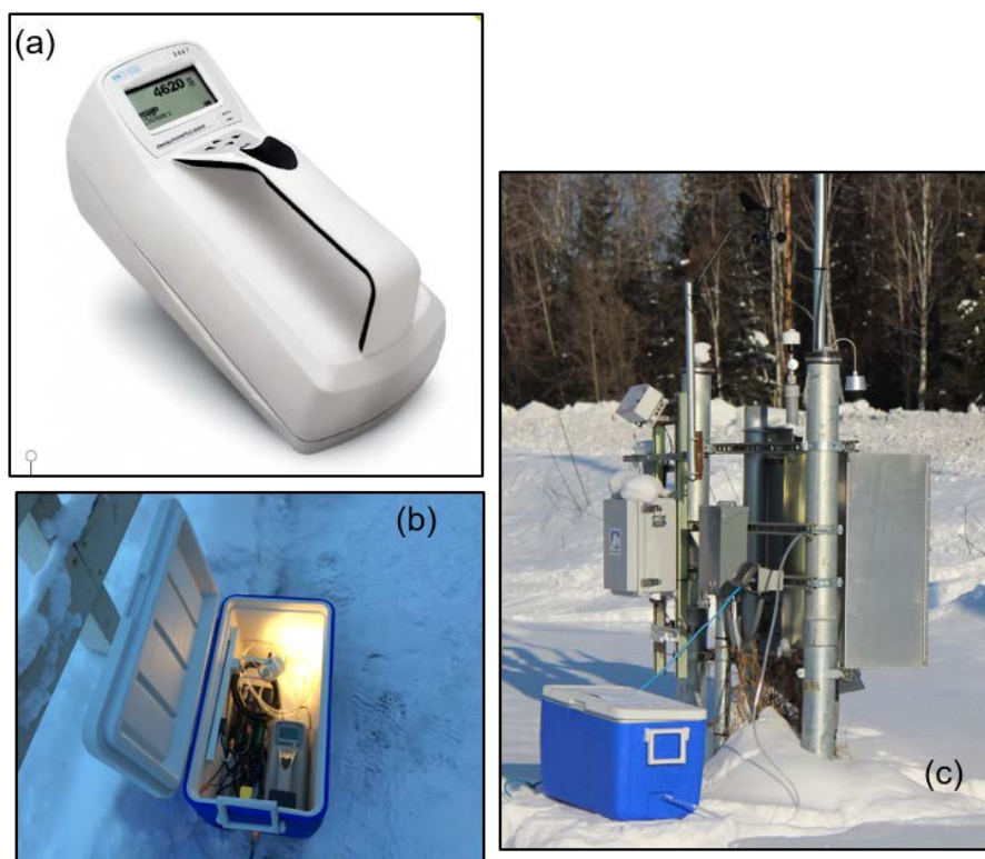
Figure 3.2 Handling of ultrafine particle counter during data collection process: (a) Condensation particle counter (CPC), Model 3007, TSI Inc.; (b) CPC housed in a cooler along with the temperature data logger and a 12V light bulb to keep the inside warm; (c) Measuring ultrafine particle concentration at RWIS station
