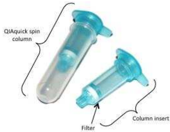
Figure 2.6: Image of QIAquick spin column used to purify DNA from successful PCR reactions. DNA is bound in the filter of the column insert when mixed with buffer PB. A wash step keeps DNA in the filter and removes excess buffers, polymerase, nucleotides and magnesium into the receptacle of the spin column. A final step adding buffer EB to the column insert elutes DNA from the filter into an Eppendorf.
