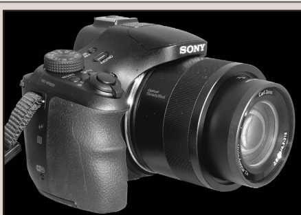
FIG. 1. The Sony DSC HX400V, one of the high-end point-and-shoot cameras we have used for 2D imaging of snake specimens. The camera has a manual focus option and a hot shoe for an external flash, as well as GPS capability.
