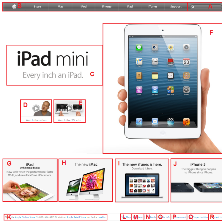
Figure 4.: The Apple page which is segmented into its elements by using the VIPS algorithm (Akpınar and Yeşilada 2013)
