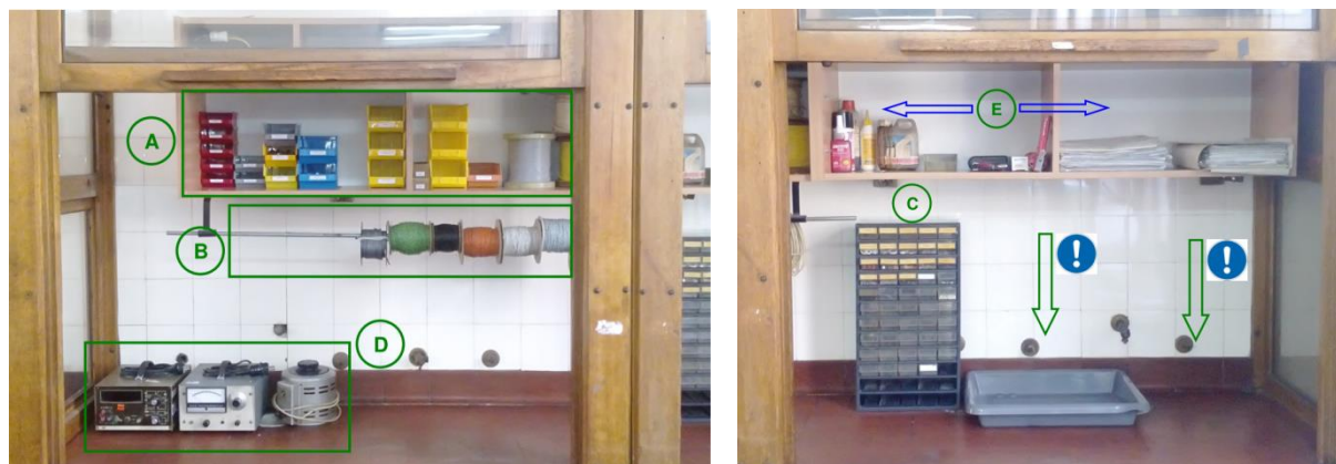
Figure 5: Presentation of set in order workplace in transmitter finalization
