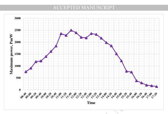
Fig. 15. Maximum power of the CPV/D module.
