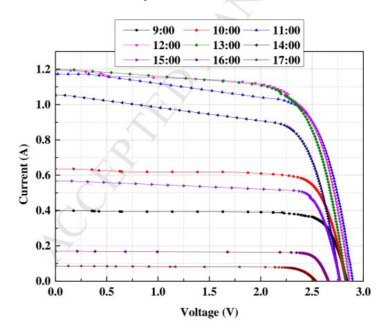
Fig. 10. I-V curves at different times of a day.
