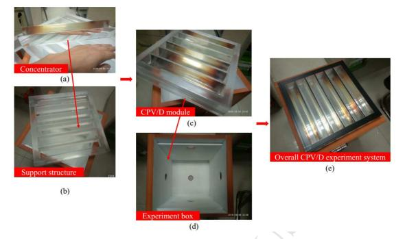
**Fig. 3.** The picture of the CPV/D system and experiment box: (a) concentrator; (b) support structure in which the concentrators are put; (c) CPV/D module; (d) experiment
