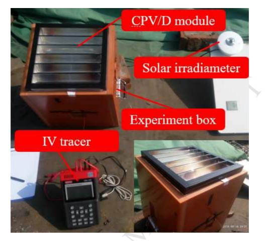
Fig. 5. The picture of the overall outdoor experiment system.
