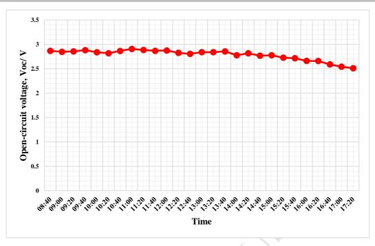
Fig. 13. Open-circuit voltage of the CPV/D module.
