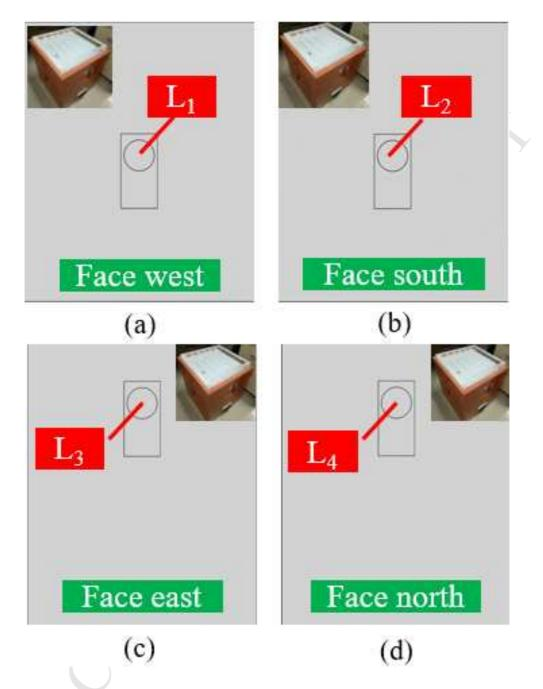
**Fig. 6.** The orientation of four facades of the experiment box and the points for the illumination test in the box ( $L_1$ ,  $L_2$ ,  $L_3$ ,  $L_4$  represent four illuminometer positions).
