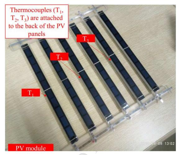
Fig.4. The PV module used in the experiment and the temperature test points for the PV
