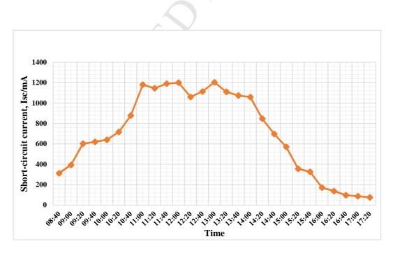
Fig. 12. Short-circuit current of the CPV/D module.
