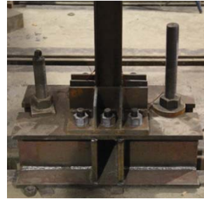
d. Column base fixture
