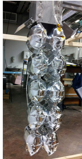
Figure 1: Prototype of 5x2cell inflatable smart structure
