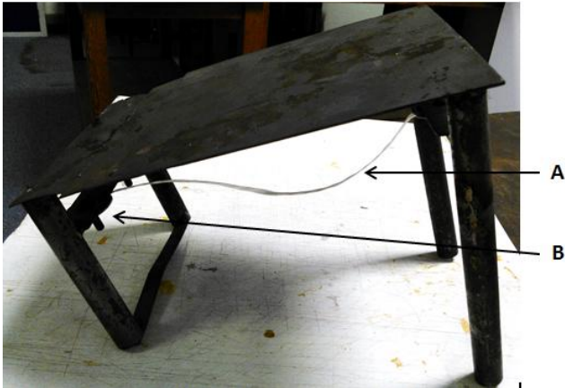
Fig.5. 2 Bundles Steel Rig. A) GF Bundle. B) Nut, bolt and washer.
