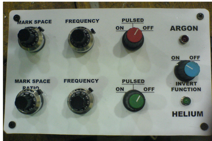
Figure 1: Electronic Gas Control Unit
