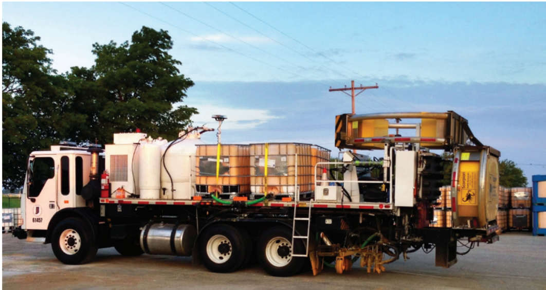
Figure 4.7 Crawfordsville paint truck modified to carry four 275-gallon paint totes.
