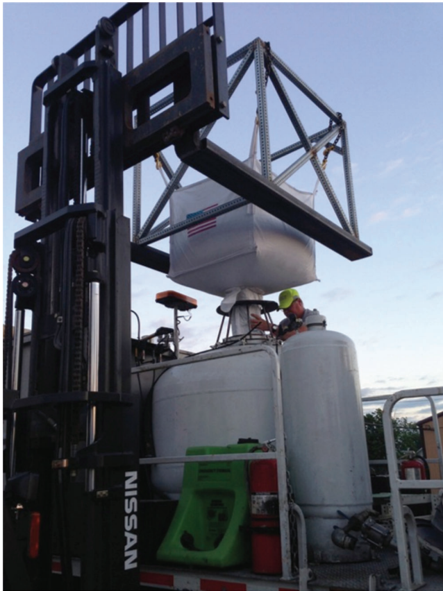
Figure 4.5 A sling bag of glass beads being gravity fed into a paint truck bead tank.
