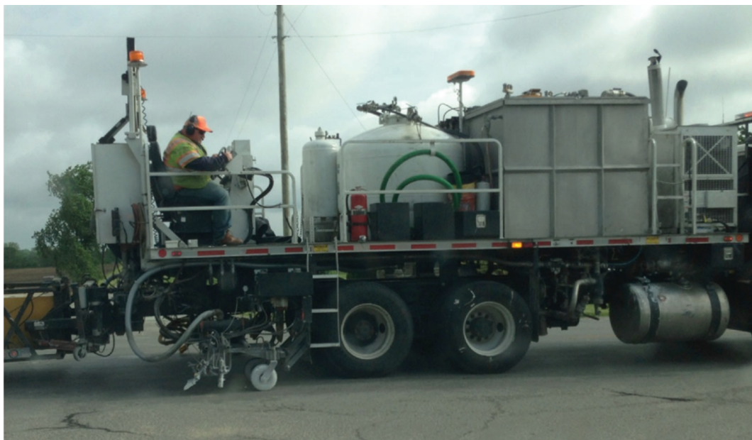
Figure 4.6 Greenfield paint truck modified with a 1,390-gallon paint tank.
