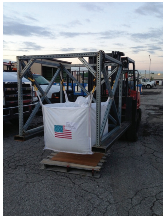
Figure 4.4 A sling bag of glass beads prepared to be lifted over a bead tank on a paint truck.
