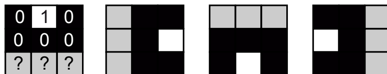
Figure 4.7: Templates used for finding end points. Each template is moved over the image, pixel-by-pixel. Where template squares are shown as set (1), the underlying pixel must also be set. Where template squares are shown as unset (0), the underlying pixel must also be unset. Grey squares can be set or unset.
