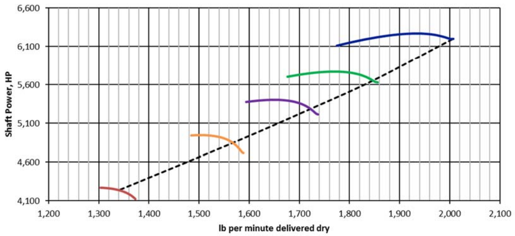
Figure 15. Case 3 Nominal Ambient Compressor Operating Map
