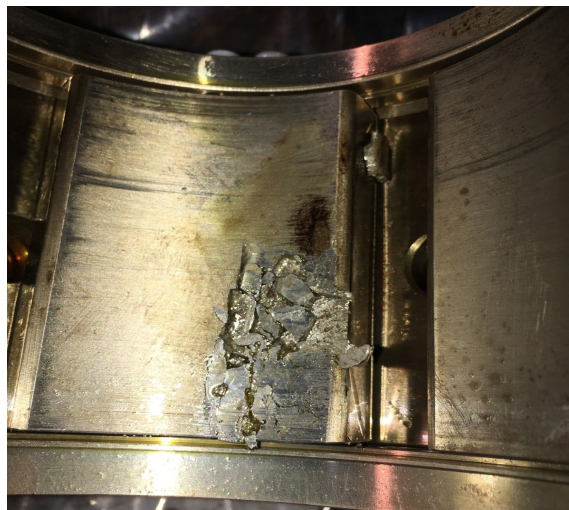
Figure 5. Observed Bearing Damages during Maintenance in November 2017
