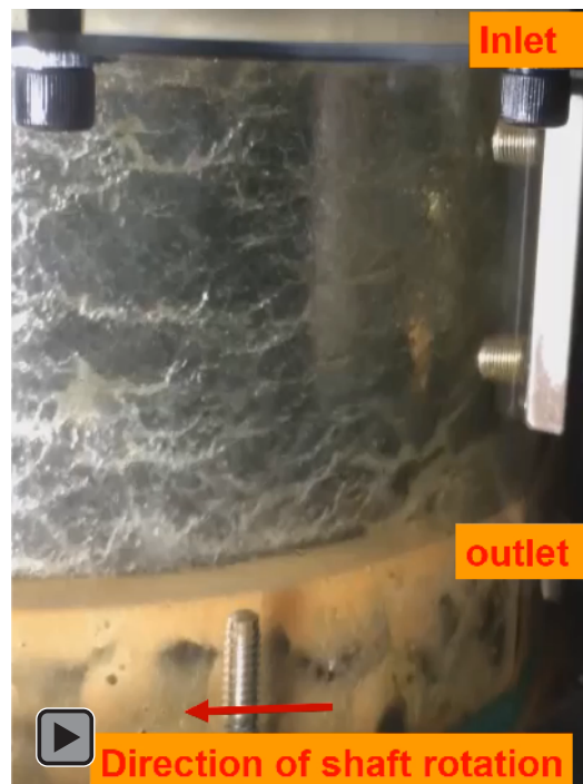
Fig. 8 Flow visualization of air-oil mixture, inlet GVF=0.9 (seal #1). Supply pressure 2 bara, discharge pressure 1 bara. Shaft speed 1.8 krpm. Videos at 60 frames/s taken with a stroboscope light with frequency = 30 Hz to freeze the shaft rotation motion. ( Click here for Web (URL) Link ).
