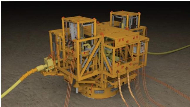
Figure 1 View of the HighBoost MPP station
