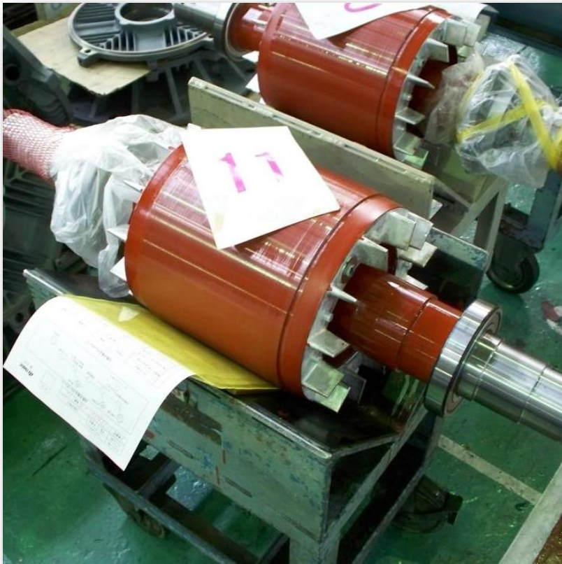
Finished Aluminum Cast Rotor with Cooling Fins (LV Motor)
