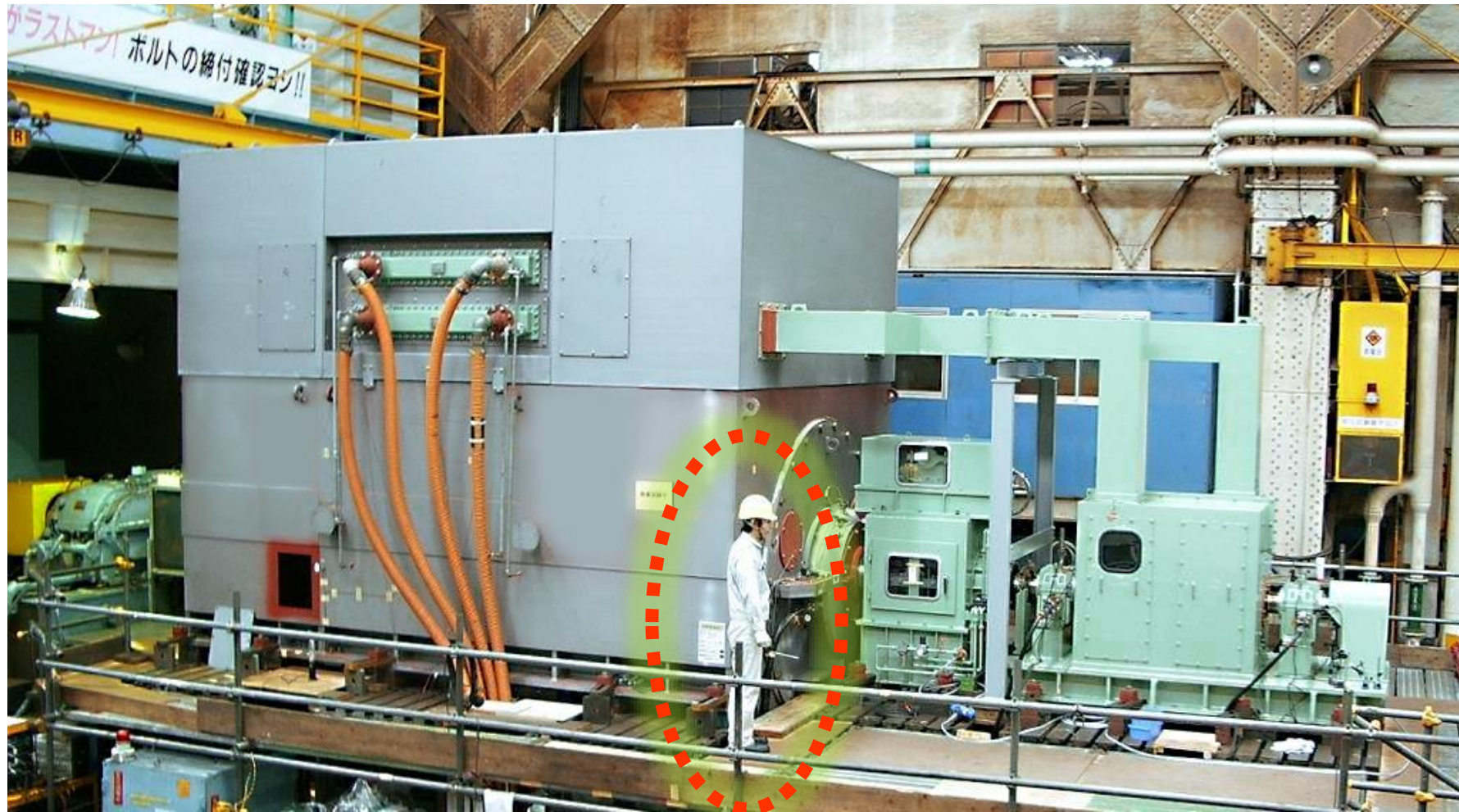
71,000HP - 2 Pole Synchronous Motor (Cylindrical Rotor)
