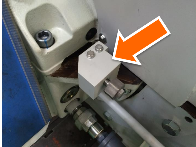
Bearing housing vibration sensor mounting provision
