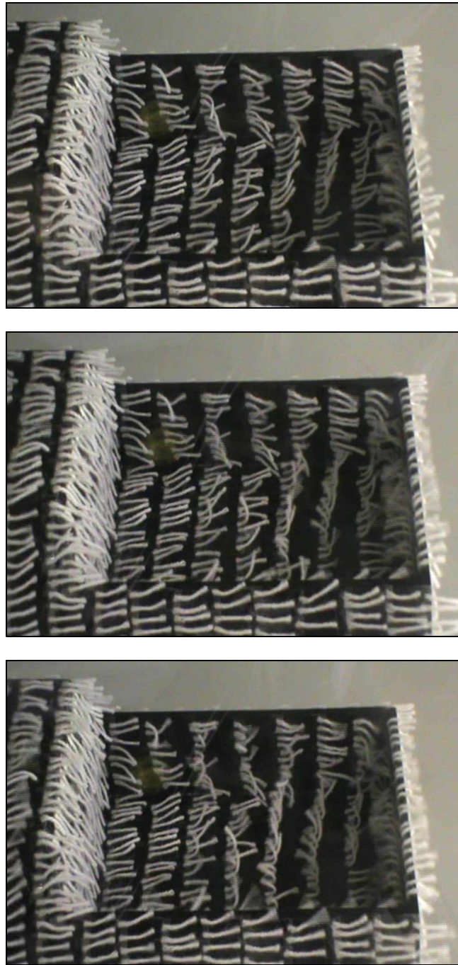
Figure 5.17 – Wall tufts on trunk for U_0 = 10 m/s (top), U_0 = 16.7 m/s (center) and U_0 = 25.0 m/s (bottom).
