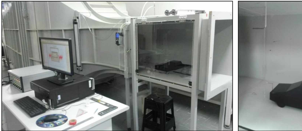
Figure 4.11 - Experimental setup (left). On detail (right) the hot-wire support and probe on position P1 and Pitot tube on test section roof.
