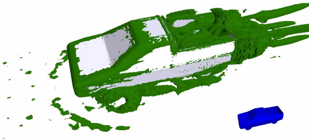
Figure 5.27 – Iso-surface of \lambda_2 = -4.0 \times 10^4 \text{ s}^{-2} for rounded model, in scale U_0 = 25 \text{ m/s} .
