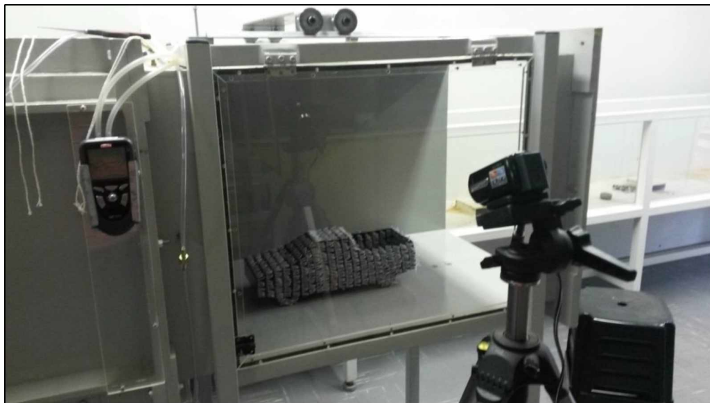
Figure 4.14 - Experimental setup for wall tufts test.
