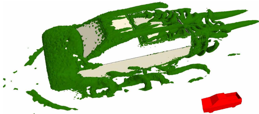
Figure 5.26 – Iso-surface of \lambda_2 = -4.0 \times 10^4 \text{ s}^{-2} for baseline model, in scale U_0 = 25 \text{ m/s} .
