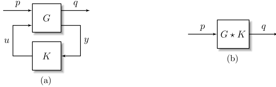
Figure 2.3: Diagram of the \mathcal{H}_\infty control problem. Figure (a) shows the LTI system G with uncertainty channel p \rightarrow q and control channel u \rightarrow y , through which we attach controller K . Figure (b) shows the same system after the loop through the control channel is closed, resulting in the system G \star K with input p and output q .
