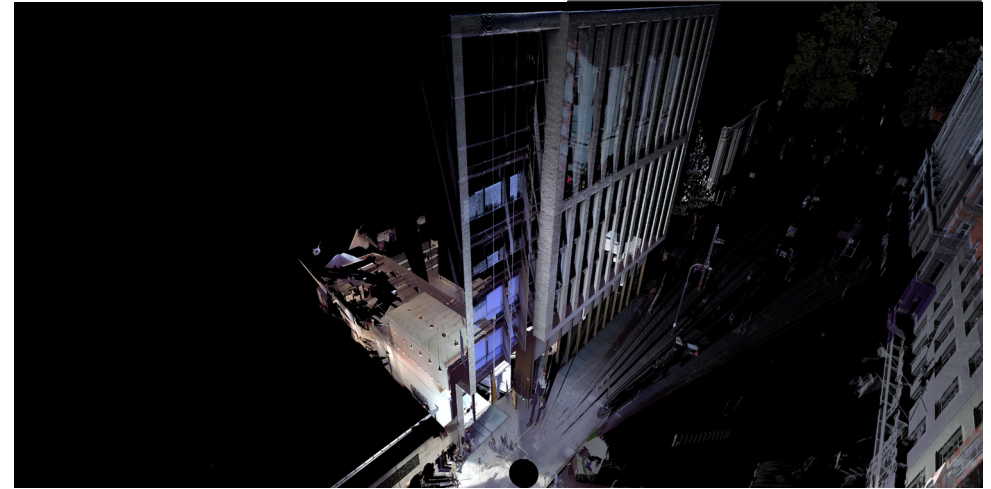
Figure 1. Aerial view of 22 Gordon Street, London, where The Bartlett School of Architecture is located. It was rendered using only one scan done outside the building during the first general class in 2017. (Source: author).
