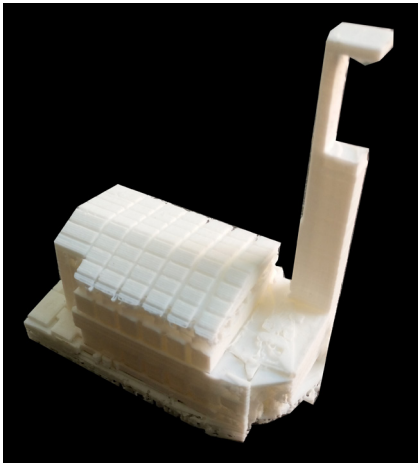
Figures 22. 3D printed models of the church based on the 3D laser scanning data of 2016. (Source: Author).
