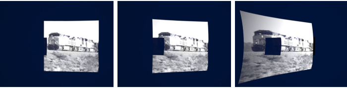
Figure 14: Stability under rotation of the lens. LuxRender renderings in the (CS/Lens) setting for the TRAIN target while rotating the lens with respect to the direction of the collimated light source ( 0^\circ / 5^\circ / 15^\circ ).
